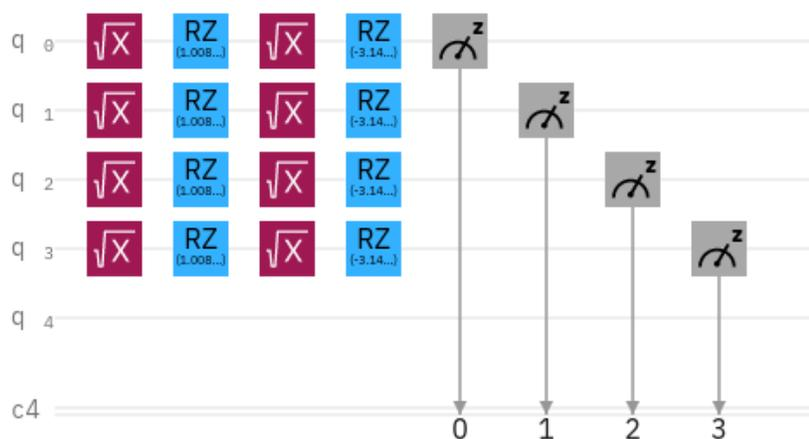
**Figure 6.10:** Quantum circuit for QPT-2 on ibm\_santiago.
