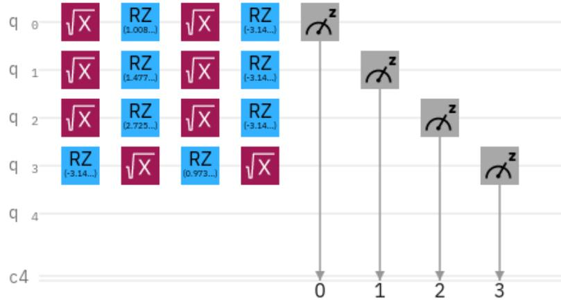
**Figure 6.9:** Quantum circuit for QPT-1 on *ibm\_santiago*.
