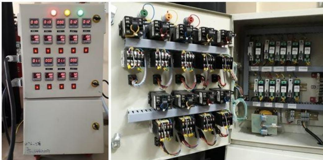
Figure 3.3. Images of the temperature controller and its electrical connection
