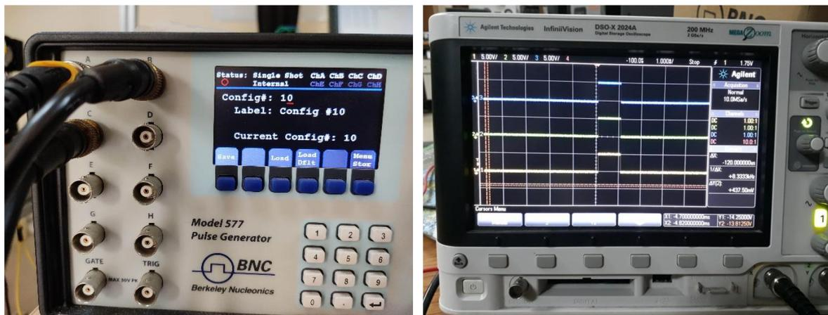
Figure 3.8. Synchronisation of different devices with a digital pulse generator and signals delay accuracy tested in an oscilloscope
