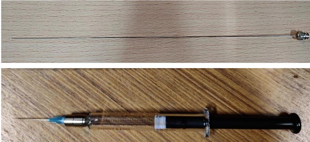
Figure 3.4. Customized lengthy needle and gas-tight syringe
