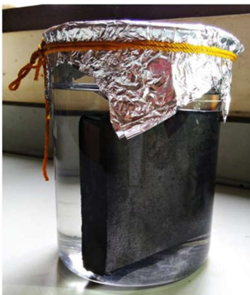
Figure 2.3 Photograph showing the setup used for the NaCl removal from carbon-NaCl composite body
