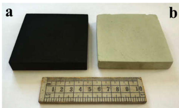
Figure 5.6 Digital photograph of (a) carbon-silicon composite foam and (b) MSiCF-2
