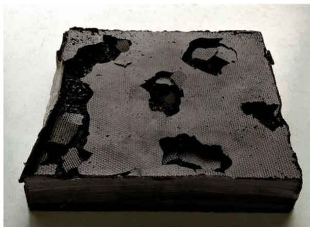
Figure 2.7 Photograph of compression-moulded body at W_{N/S} of 0.5 showing large voids
