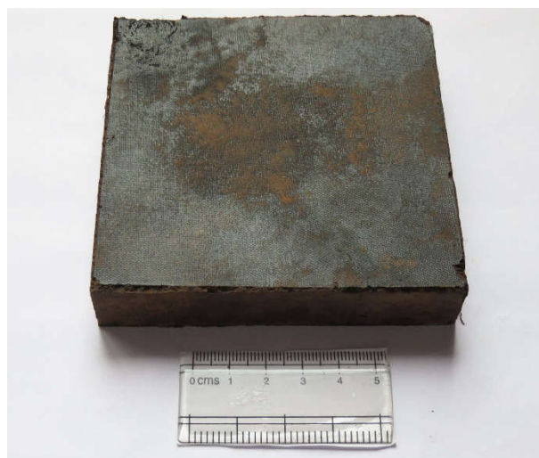
Figure 2.6 Photographic image of sucrose polymer-NaCl composite body obtained after compression moulding and setting
