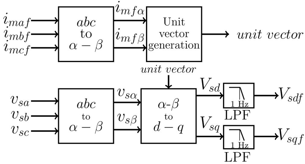
**Figure 2.14:** The block diagram showing the transformation of the fundamental component of motor currents ( $i_{maf}, i_{mbf}$  and  $i_{mcf}$ ) and the CSI terminal voltages ( $v_{sa}, v_{sb}$  and  $v_{sc}$ ) from abc to d-q frame of reference
