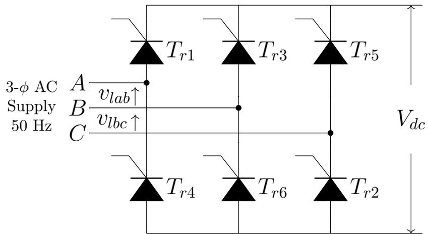
**Figure 2.2:** Line commutated SCR based rectifier.
