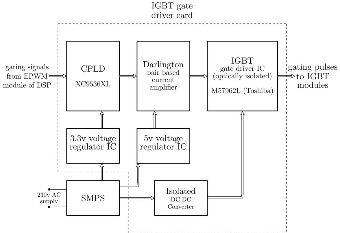
**Figure 5.5:** Block diagram of IGBT gate driver circuit.
