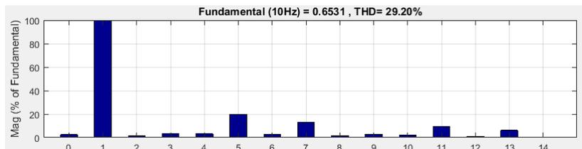
**Figure 3.26:** Harmonic spectrum of motor current shown in Fig.3.25 with single CSI operation: X-axis (Harmonic order). Y-axis: (Magnitude in % of fundamental).
