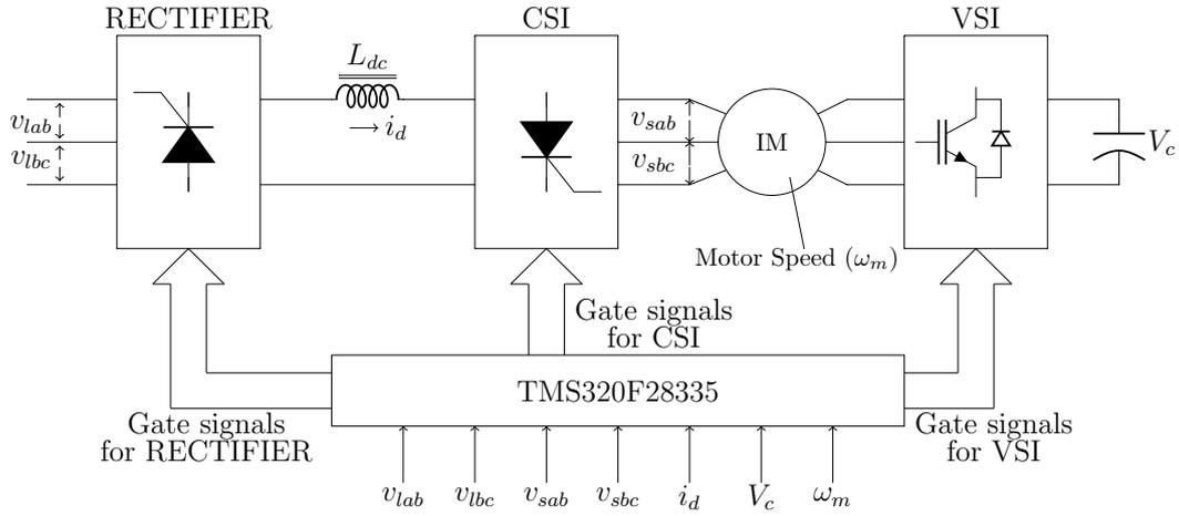
**Figure 2.17:** Implementation of the overall control scheme of the proposed drive system.
