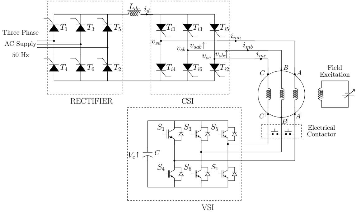
**Figure 4.2:** Complete Power Circuit diagram of the proposed scheme.
