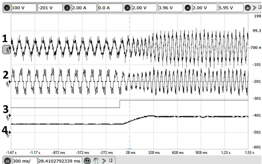
**Figure 3.23:** Experimental results: Step change in motor speed from 300 RPM to 600 RPM: X-axis: 300 ms/div. Ch-1: A-phase stator voltage of motor (Y-axis: 100 V/div). Ch-2: A-phase motor current (Y-axis: 2 A/div). Ch-3: Motor speed reference (Y-axis: 666 rpm/div). Ch-4: Actual motor speed (Y-axis: 666 rpm/div).
