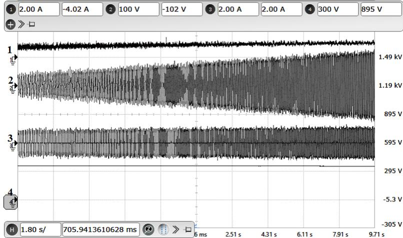
**Figure 2.26:** Experimental results: Motor accelerated from 300 RPM to 1000 RPM : X-axis: 1.8 s/div. Ch-1: DC link current (Y-axis: 2 A/div). Ch-2: A-phase stator voltage(Y-axis: 100 V/div). Ch-3: A-phase motor current (Y-axis: 2 A/div). Ch-4: VSI capacitor voltage (Y-axis: 300 V/div).
