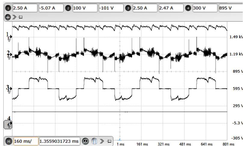
**Figure 2.29:** Experimental results: Motor operation at 70 RPM : X-axis: 160 ms/div. Ch-1: DC link current (Y-axis: 2.5 A/div). Ch-2: A-phase stator voltage(Y-axis: 100 V/div). Ch-3: A-phase motor current (Y-axis: 2.5 A/div). Ch-4: VSI capacitor voltage (Y-axis: 300 V/div).
