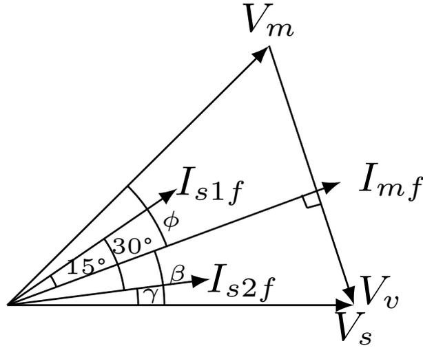
**Figure 3.8:** Phasor diagram showing CSI terminal voltage ( $V_s$ ), motor voltage ( $V_m$ ), VSI output voltage ( $V_v$ ) and fundamental components of motor current ( $I_{mf}$ ), CSI-1 current ( $I_{s1f}$ ), CSI-2 current ( $I_{s2f}$ ).
