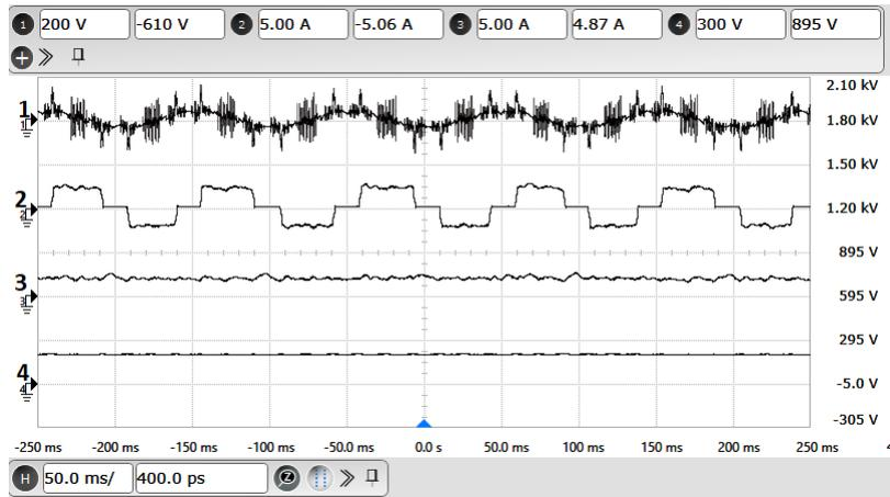
**Figure A.4:** Experimental results with single CSI configuration: Motor operation at 300 RPM : X-axis: 50 ms/div. Ch-1: A-phase stator voltage (Y-axis: 200 V/div). Ch-2: A-phase motor current (Y-axis: 5 A/div) . Ch-3: DC link current (Y-axis: 5 A/div) . Ch-4: VSI capacitor voltage (Y-axis: 300 V/div).
