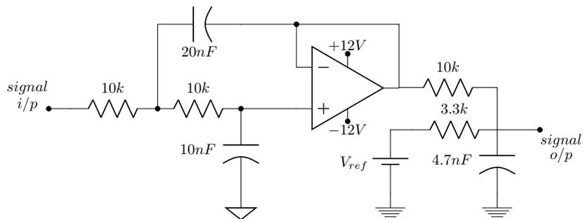
**Figure 5.7:** Circuit schematic of Sallen-Key filter.
