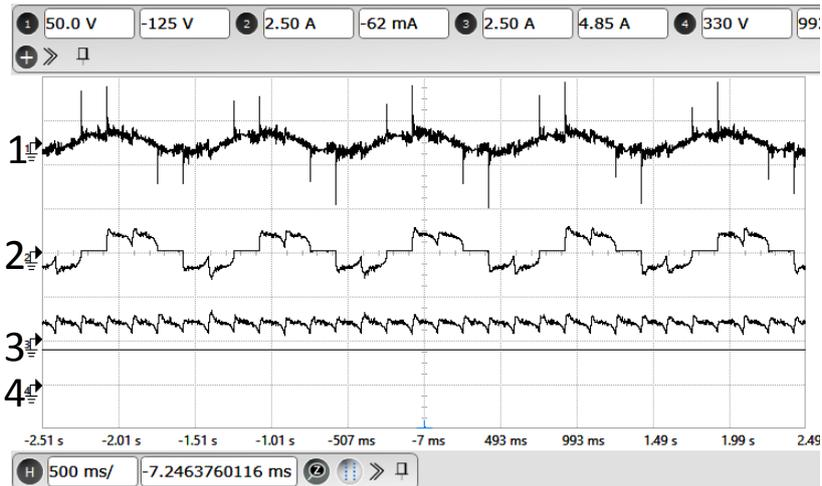
**Figure 4.7:** Experimental result at 30 RPM of motor operation: X-axis: 500 ms/div. Ch:1. Motor voltage (Y-axis: 50 V/div.). Ch:2. Motor current (Y-axis: 2.5 A/div.). Ch:3. DC-link current (Y-axis: 2.5 A/div.).Ch:4. VSI capacitor voltage (Y-axis: 330 V/div.).
