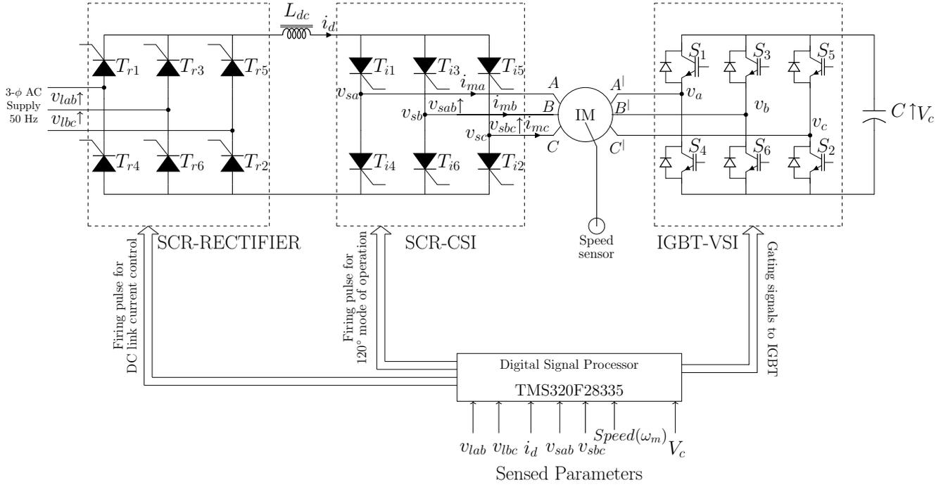
**Figure 2.1:** Power circuit diagram of the proposed scheme.
