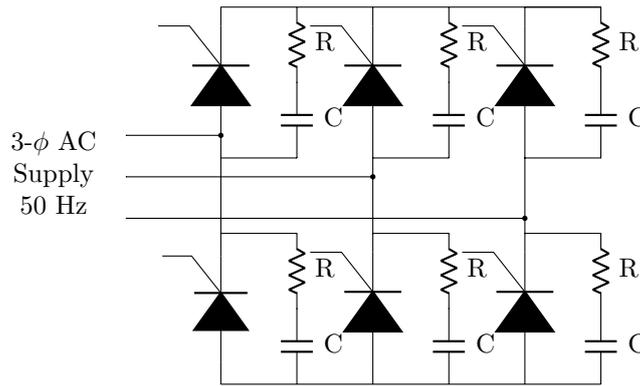
**Figure 5.1:** Power circuit diagram of SCR based rectifier.
