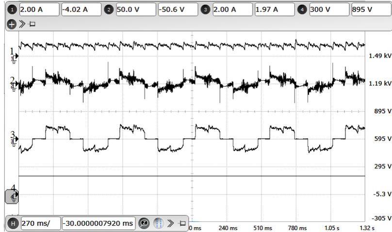
**Figure 2.28:** Experimental results: Motor operation at 50 RPM : X-axis: 270 ms/div. Ch-1: DC link current (Y-axis: 2 A/div). Ch-2: A-phase stator voltage(Y-axis: 50 V/div). Ch-3: A-phase motor current (Y-axis: 2 A/div). Ch-4: VSI capacitor voltage (Y-axis: 300 V/div).
