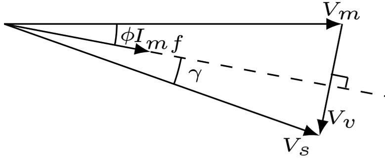
**Figure 2.10:** System phasor diagram representing the motor voltage ( $V_m$ ), VSI voltage ( $V_v$ ) and the CSI terminal voltage ( $V_s$ )
