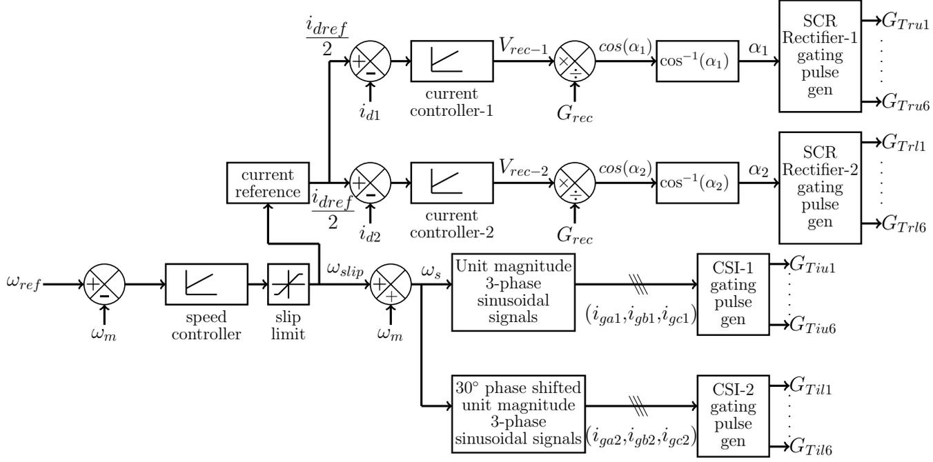
**Figure 3.9:** Control scheme of multilevel CSI.
