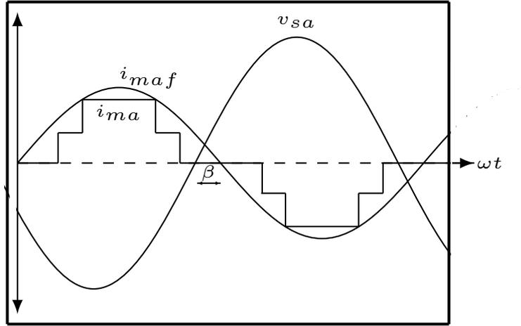
**Figure 3.13:** CSI terminal voltage ( $v_{sa}$ ), machine current ( $i_{ma}$ ) and its fundamental component ( $i_{maf}$ ) during regeneration.
