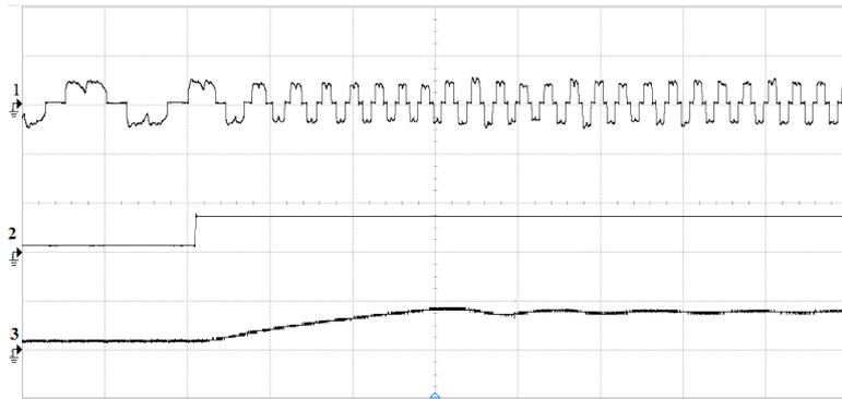
**Figure 2.27:** Experimental results: Step change in motor speed from 100 RPM to 500 RPM: X-axis: 200 ms/div. Ch-1: A-phase motor current (Y-axis: 2 A/div). Ch-2: Motor speed reference (Y-axis: 666 rpm/div). Ch-3: Actual motor speed (Y-axis: 666 rpm/div).
