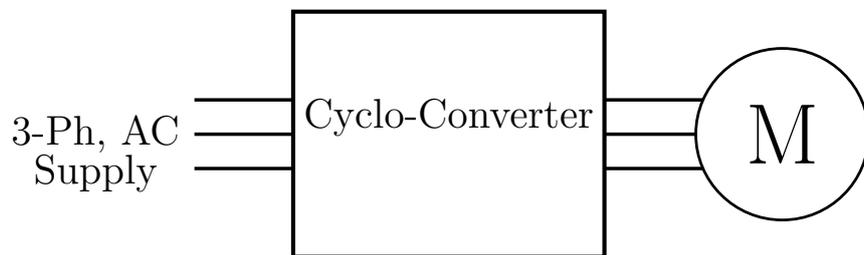
**Figure 1.7:** Block diagram of cyclo-converter based drive.
