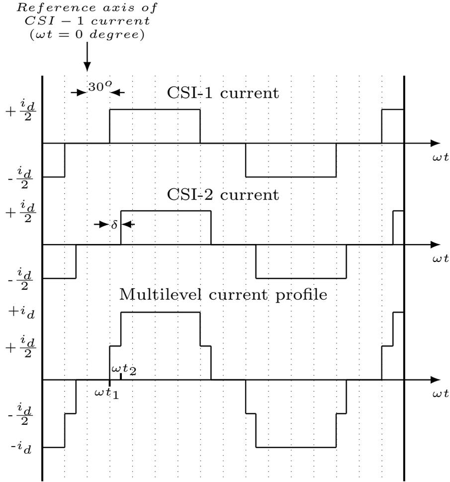
**Figure 3.2:** Multilevel current waveform with  $\delta$  angle phase shifted operation of CSIs.
