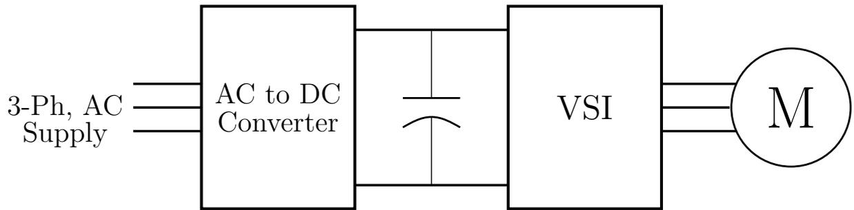
**Figure 1.2:** Block diagram of VSI fed drive.
