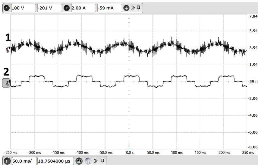
**Figure 3.25:** Experimental results: Motor operation at 300 RPM with single CSI: X-axis: 50 ms/div. Ch-1: A-phase stator voltage of motor (Y-axis: 100 V/div). Ch-2: A-phase motor current (Y-axis: 2 A/div).
