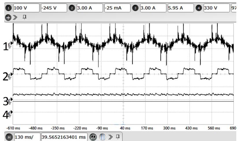
**Figure 4.10:** Experimental result at 150 RPM of motor operation: X-axis: 130 ms/div. Ch:1. Motor voltage (Y-axis: 100 V/div.). Ch:2. Motor current (Y-axis: 3 A/div.). Ch:3. DC-link current (Y-axis: 3 A/div.).Ch:4. VSI capacitor voltage (Y-axis: 330 V/div.).
