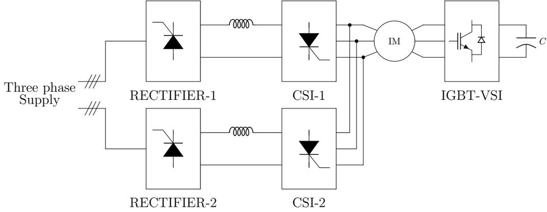
**Figure 3.1:** Block diagram of the proposed load commutated multilevel CSI scheme for open-end winding induction motor drives.
