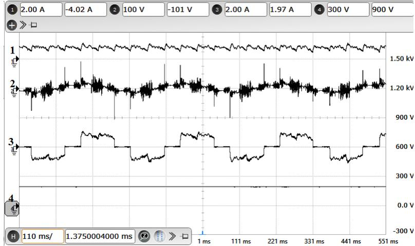
**Figure 2.30:** Experimental results: Motor operation at 100 RPM : X-axis: 110 ms/div. Ch-1: DC link current (Y-axis: 2 A/div). Ch-2: A-phase stator voltage(Y-axis: 100 V/div). Ch-3: A-phase motor current (Y-axis: 2 A/div). Ch-4: VSI capacitor voltage (Y-axis: 300 V/div).
