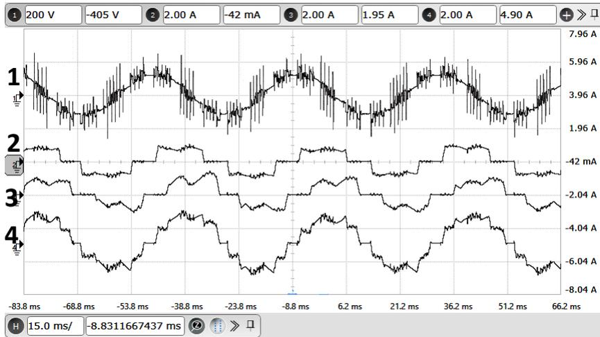
**Figure 3.17:** Experimental results : Motoring operation at 750 RPM: X-axis: 15ms/div. Ch-1: A-phase stator voltage of motor (Y-axis: 200 V/div). Ch-2: A-phase CSI-1 current (Y-axis: 2 A/div). Ch-3: A-phase CSI-2 current (Y-axis: 2 A/div). Ch-4: A-phase motor current (Y-axis: 2 A/div).
