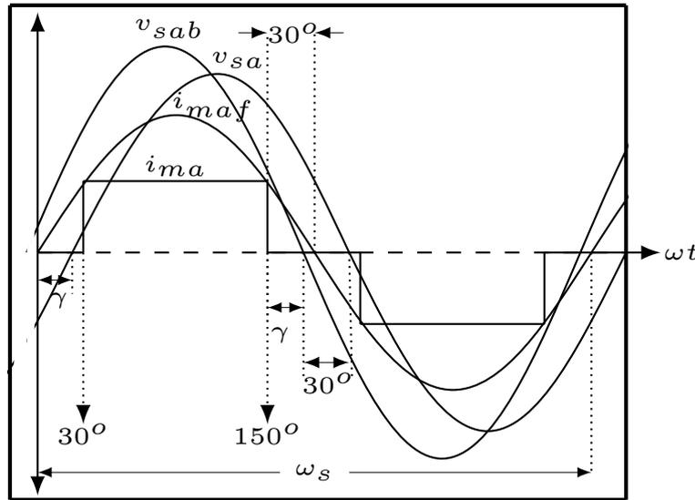
**Figure 2.8:** CSI terminal voltage ( $v_{sa}$ ), CSI line voltage ( $v_{sab}$ ), motor current  $i_{ma}$  and its fundamental component ( $i_{maf}$ ) waveforms.
