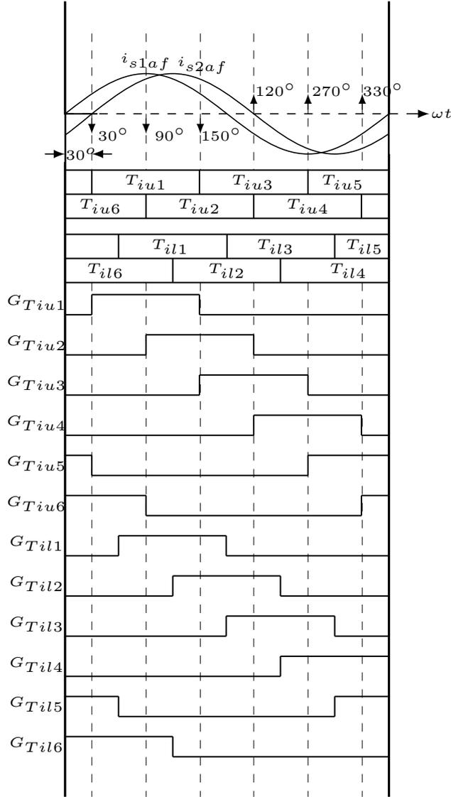
**Figure 3.6:** SCR conduction period and their gating pulses of CSI-1 and CSI-2.
