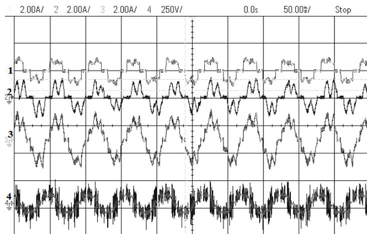
**Figure A.8:** Experimental results with multilevel CSI configuration : Motoring operation at 500 RPM: X-axis: 50ms/div. Ch-1: A-phase CSI-1 current (Y-axis: 2 A/div). Ch-2: A-phase CSI-2 current (Y-axis: 2 A/div) . Ch-3: A-phase motor current (Y-axis: 2 A/div). Ch-4: A-phase stator voltage of motor (Y-axis: 250 V/div).
