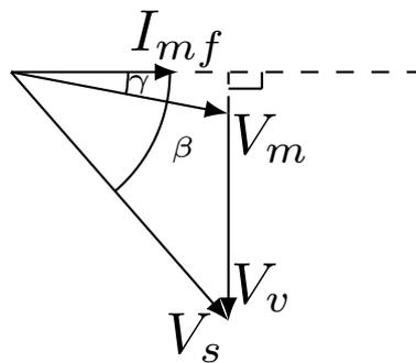
**Figure 4.3:** System phasor diagram with VSI in operation.
