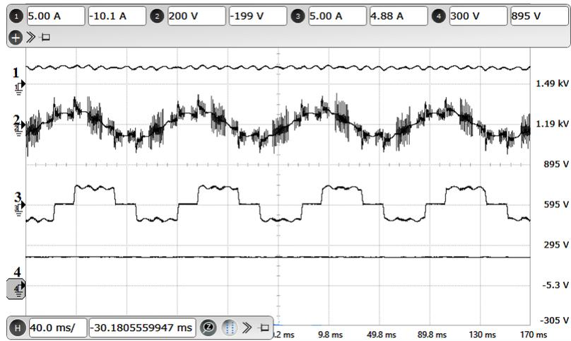
**Figure 2.25:** Experimental results: Motor operation at 300 RPM in loaded condition : X-axis: 40 ms/div. Ch-1: DC link current (Y-axis: 5 A/div). Ch-2: A-phase stator voltage(Y-axis: 200 V/div). Ch-3: A-phase motor current (Y-axis: 5 A/div). Ch-4: VSI capacitor voltage (Y-axis: 300 V/div).
