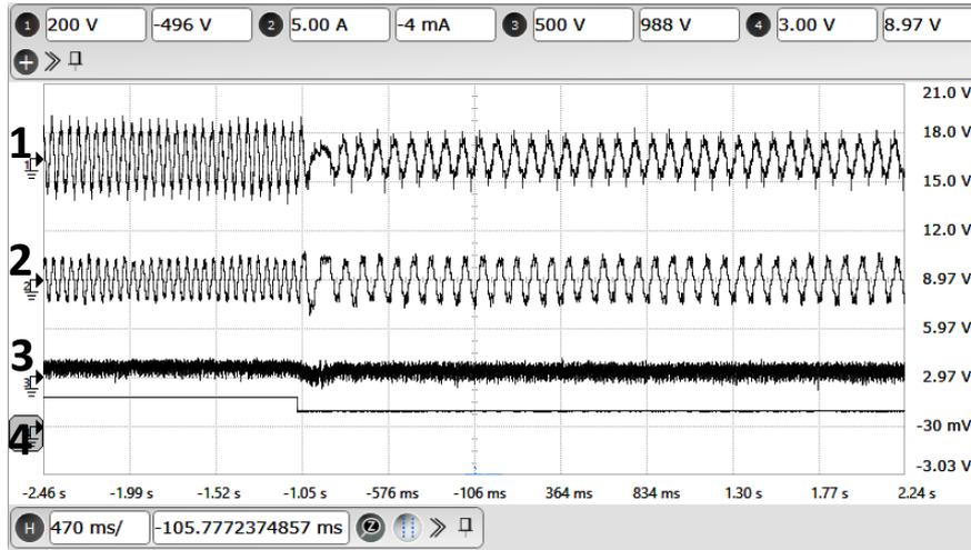
**Figure 3.29:** Experimental results: Regenerative braking of the drive during step change in motor speed from 600 RPM to 300 RPM : X-axis: 470 ms/div. Ch-1: A-phase stator voltage of motor (Y-axis: 200 V/div). Ch-2: A-phase motor current (Y-axis: 5 A/div). Ch-3: DC link voltage of Rectifier-1 (Y-axis: 500 V/div). Ch-4: Motor speed reference (Y-axis: 333 rev/min/div).
