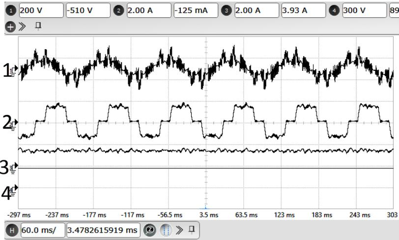
**Figure 4.11:** Experimental result at 300 RPM of motor operation: X-axis: 60 ms/div. Ch:1. Motor voltage (Y-axis: 200 V/div.). Ch:2. Motor current (Y-axis: 2 A/div.). Ch:3. DC-link current (Y-axis: 2 A/div.).Ch:4. VSI capacitor voltage (Y-axis: 300 V/div.).
