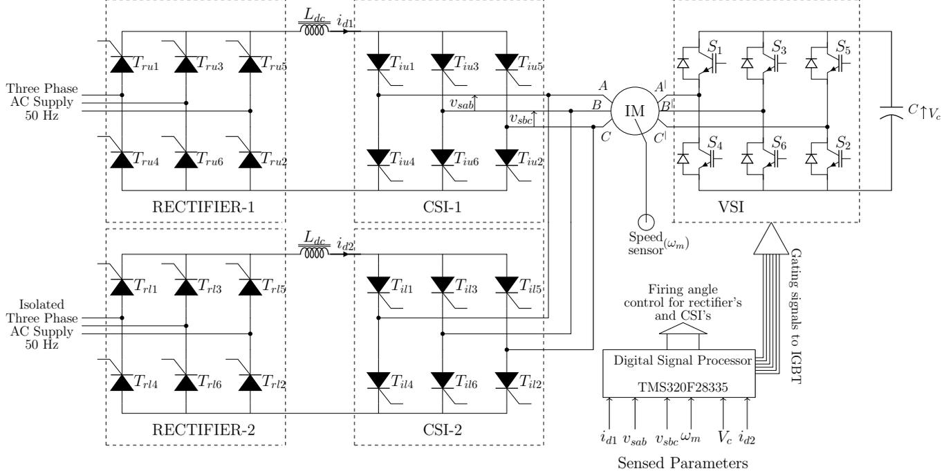
**Figure 3.4:** Power circuit diagram of the proposed load commutated multilevel CSI scheme for open-end winding induction motor drive.
