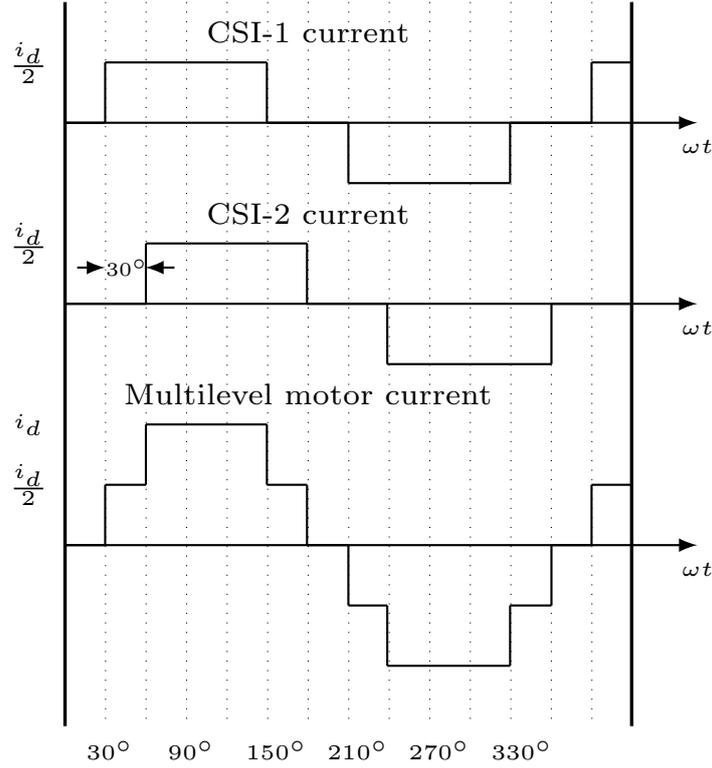
**Figure 3.5:** Motor current and CSI current waveforms.
