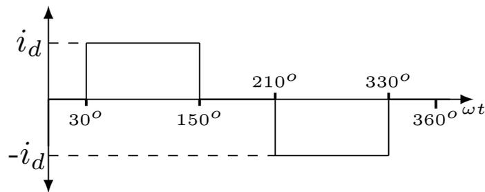
**Figure 2.6:** Per-phase CSI current or motor current.
