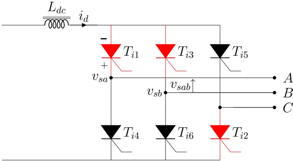
**Figure 2.9:** Circuit state at the commutation of A-phase top SCR  $T_{i1}$ .
