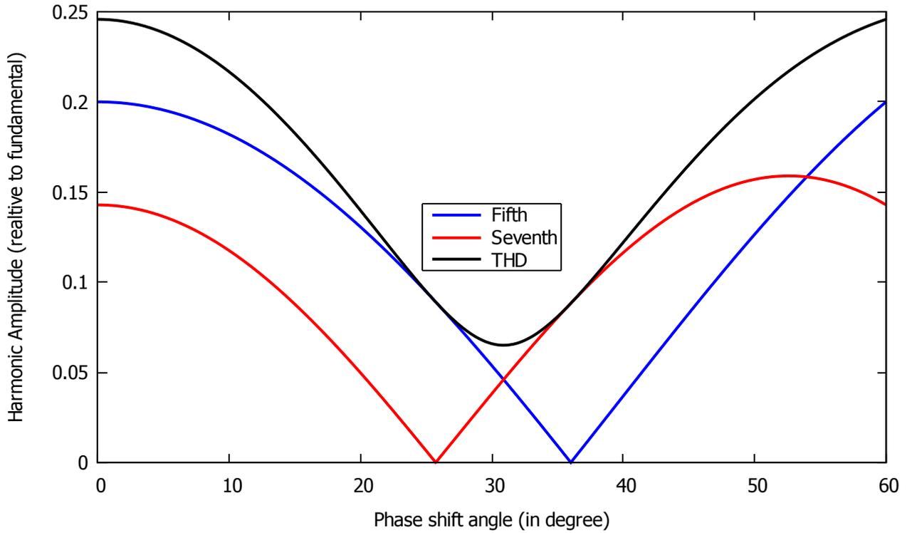
**Figure 3.3:** Variation in 5<sup>th</sup> harmonic , 7<sup>th</sup> harmonic and the THD of motor current with respect to the phase shift angle  $\delta$  between the output currents of CSI-1 and CSI-2.
