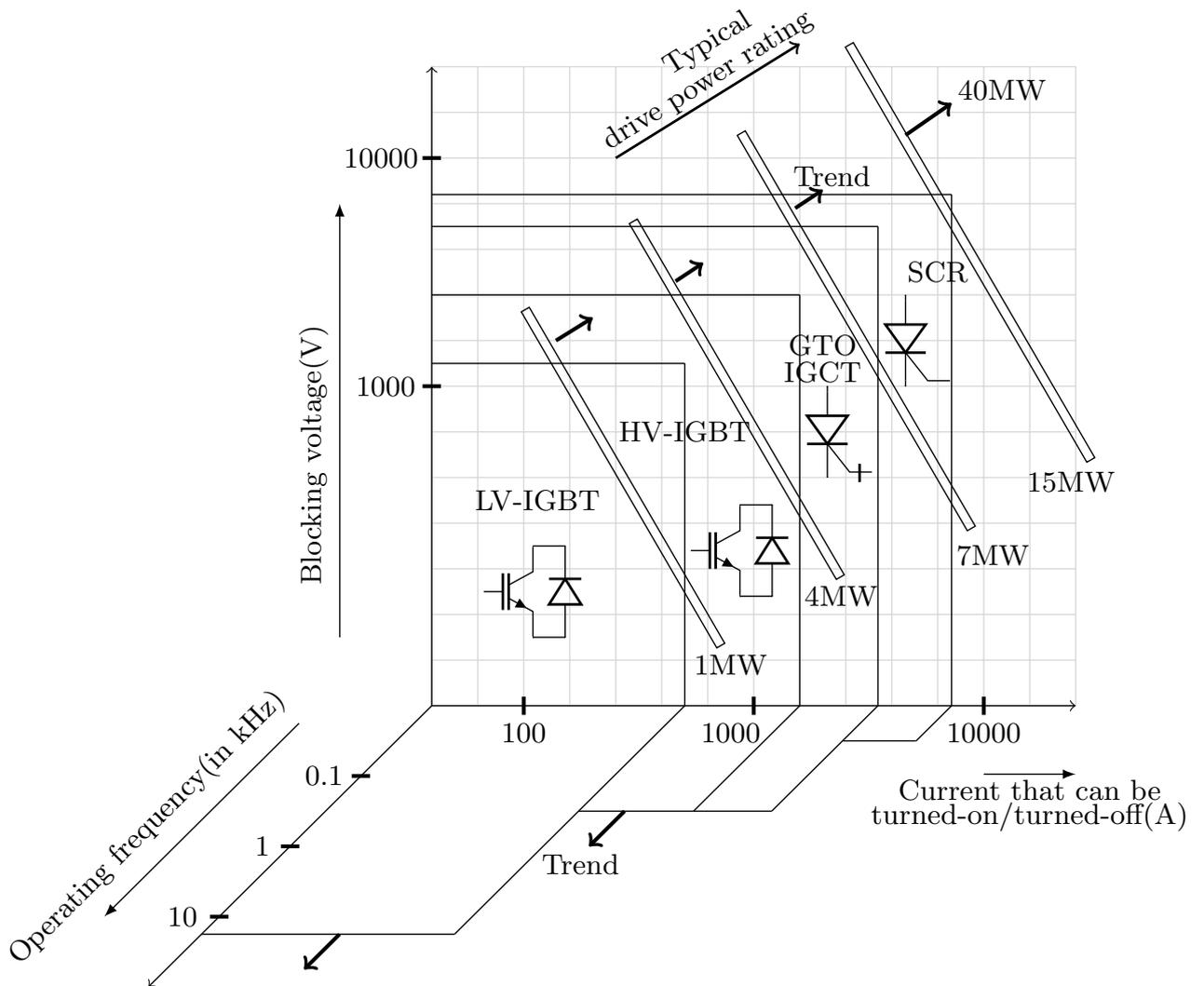
**Figure 1.1:** Power semiconductor devices and their ratings.
