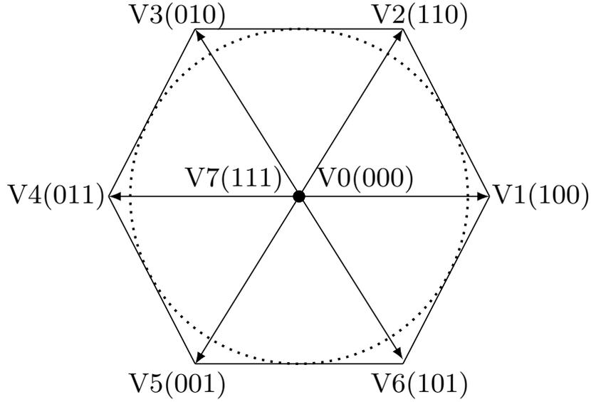
**Figure 1.6:** Voltage space vector structure of a three phase inverter.
