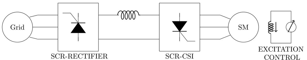
**Figure 1.9:** Block diagram of load commutated inverter fed synchronous motor drive.
