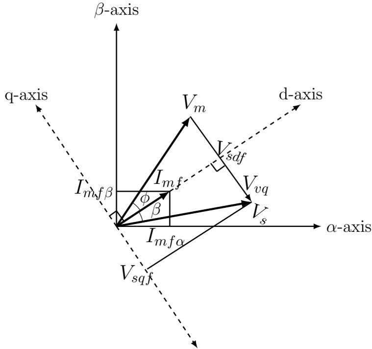
**Figure 3.11:** Phasor diagram showing the orientation of d-q axes, fundamental component of motor current ( $I_{mf}$ ) and CSI terminal voltage ( $V_s$ ).
