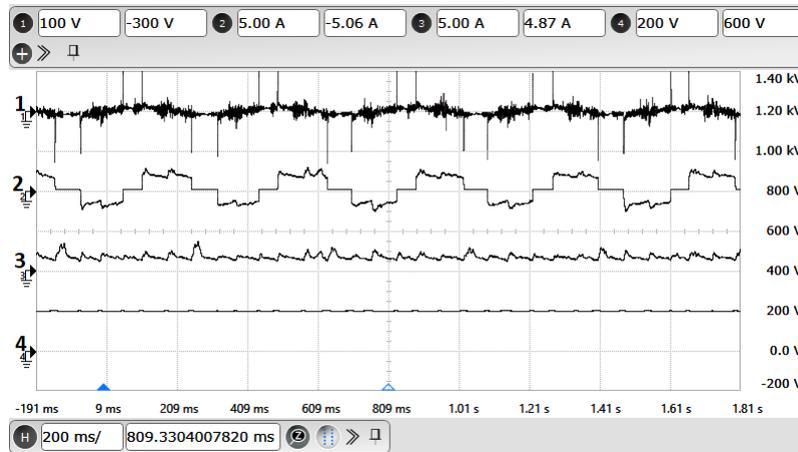
**Figure A.6:** Experimental results with single CSI configuration: Motor operation at 150 RPM : X-axis: 200 ms/div. Ch-1: A-phase stator voltage (Y-axis: 100 V/div). Ch-2: A-phase motor current (Y-axis: 5 A/div) . Ch-3: DC link current (Y-axis: 5 A/div) . Ch-4: VSI capacitor voltage (Y-axis: 200 V/div).
