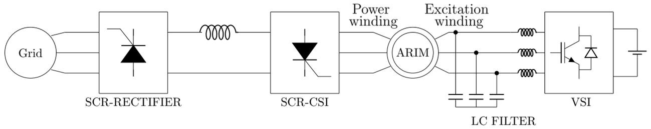
**Figure 1.13:** Block diagram of a hybrid CSI-VSI based configuration for load commutated Active Reactive Induction Machine.
