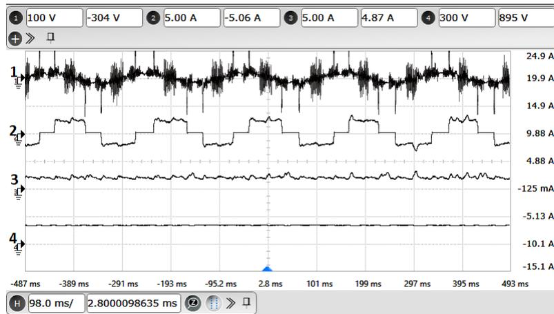
**Figure A.5:** Experimental results with single CSI configuration: Motor operation at 150 RPM : X-axis: 98 ms/div. Ch-1: A-phase stator voltage (Y-axis: 100 V/div). Ch-2: A-phase motor current (Y-axis: 5 A/div) . Ch-3: DC link current (Y-axis: 5 A/div) . Ch-4: VSI capacitor voltage (Y-axis: 300 V/div).
