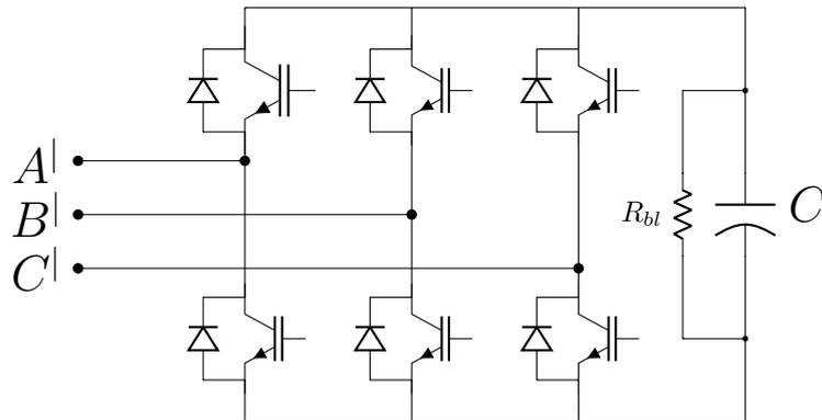
**Figure 5.4:** Power circuit diagram of IGBT based VSI.
