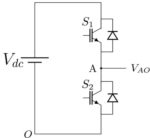
**Figure 1.4:** Single leg of three-phase inverter with high side switch as ' $S_1$ ' and low side switch as ' $S_2$ '.
