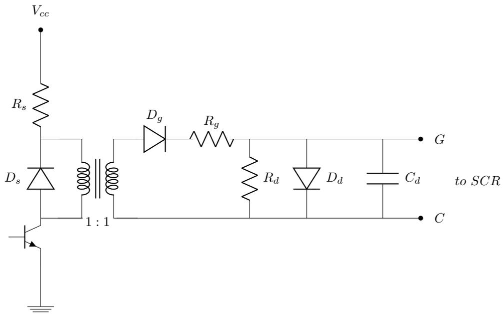
**Figure 5.3:** Circuit schematic of SCR gate driver.
