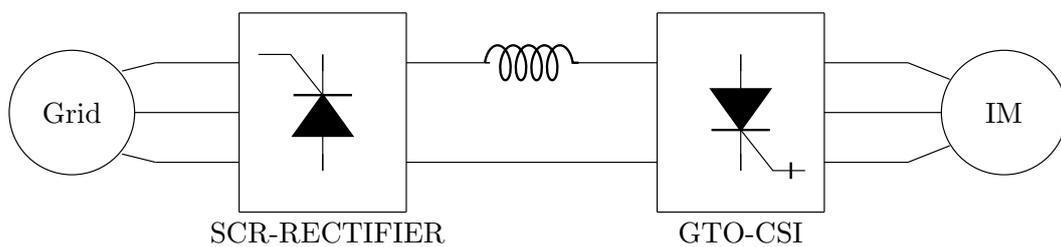
**Figure 1.10:** Block diagram of GTO based CSI fed induction motor drive.
