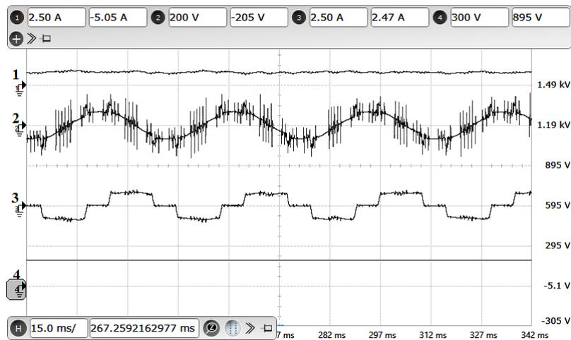
**Figure 2.21:** Experimental results: Motor operation at 750 RPM : X-axis: 15 ms/div. Ch-1: DC link current (Y-axis: 2.5 A/div). Ch-2: A-phase stator voltage(Y-axis: 200 V/div). Ch-3: A-phase motor current (Y-axis: 2.5 A/div). Ch-4: VSI capacitor voltage (Y-axis: 300 V/div).
