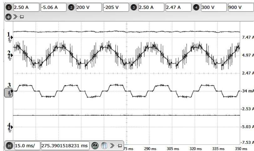
**Figure 2.23:** Experimental results: Motor operation at 1000 RPM : X-axis: 15 ms/div. Ch-1: DC link current (Y-axis: 2.5 A/div). Ch-2: A-phase stator voltage(Y-axis: 200 V/div). Ch-3: A-phase motor current (Y-axis: 2.5 A/div). Ch-4: VSI capacitor voltage (Y-axis: 300 V/div).
