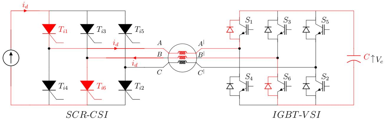
**Figure 2.18:** Pre-charging scheme of the VSI capacitor
