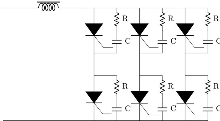
**Figure 5.2:** Power circuit diagram of Load commutated SCR based CSI.
