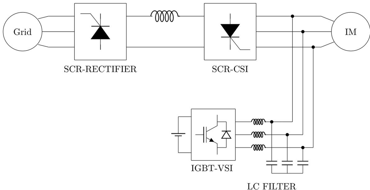
**Figure 1.12:** Block diagram of the hybrid scheme of load commutated SCR based induction motor drive with shunt connected IGBT based VSI.
