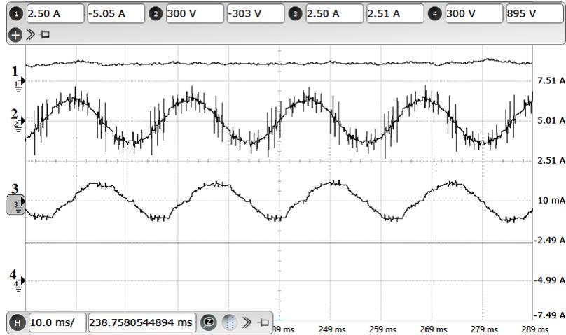
**Figure 2.24:** Experimental results: Motor operation at 1300 RPM : X-axis: 10 ms/div. Ch-1: DC link current (Y-axis: 2.5 A/div). Ch-2: A-phase stator voltage(Y-axis: 300 V/div). Ch-3: A-phase motor current (Y-axis: 2.5 A/div). Ch-4: VSI capacitor voltage (Y-axis: 300 V/div).
