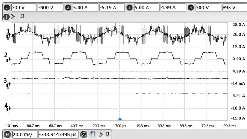
**Figure A.3:** Experimental results with single CSI configuration: Motor operation at 750 RPM : X-axis: 20 ms/div. Ch-1: A-phase stator voltage (Y-axis: 300 V/div). Ch-2: A-phase motor current (Y-axis: 5 A/div) . Ch-3: DC link current (Y-axis: 5 A/div) . Ch-4: VSI capacitor voltage (Y-axis: 300 V/div).
