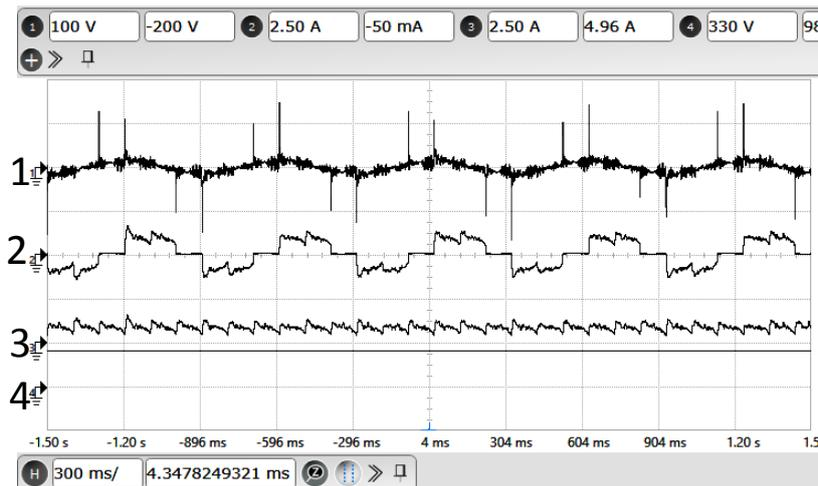
**Figure 4.8:** Experimental result at 50 RPM of motor operation: X-axis: 300 ms/div. Ch:1. Motor voltage (Y-axis: 100 V/div.). Ch:2. Motor current (Y-axis: 2.5 A/div.). Ch:3. DC-link current (Y-axis: 2.5 A/div.).Ch:4. VSI capacitor voltage (Y-axis: 330 V/div.).
