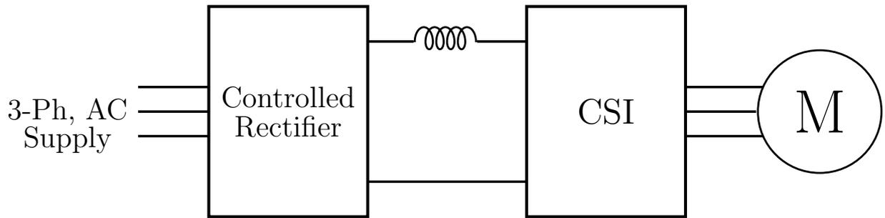
**Figure 1.8:** Block diagram of CSI fed AC motor drives.
