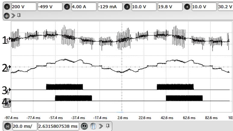
**Figure 3.19:** Experimental results : 300 RPM (or 10 Hz) motor operation: X-axis: 20 ms/div. Ch-1: A-phase stator voltage of motor (Y-axis: 200 V/div). Ch-2: A-phase motor current (Y-axis: 4 A/div). Ch-3: CSI-1 A-phase top SCR triggering pulse (Y-axis: 10 V/div). Ch-4: CSI-2 A-phase top SCR triggering pulse (Y-axis: 10 V/div).
