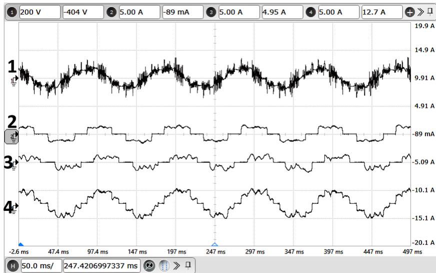
**Figure 3.20:** Experimental results: Motoring operation at 300 RPM with load: X-axis: 50 ms/div. Ch-1: A-phase stator voltage of motor (Y-axis: 200 V/div). Ch-2: A-phase CSI-1 current (Y-axis: 5 A/div). Ch-3: A-phase CSI-2 current (Y-axis: 5 A/div). Ch-4: A-phase motor current (Y-axis: 5 A/div).
