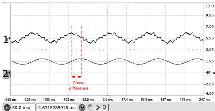
**Figure 3.21:** Experimental results: X-axis: 50 ms/div. Ch-1: A-phase motor current (Y-axis: 5 A/div). Ch-2: A-phase modulating voltage of VSI captured using unipolar DAC of DSP, the bipolar modulating signal is DC shifted by a unit division (Y-axis: 0.5 unit/div) .
