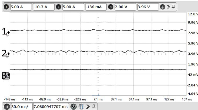
**Figure 3.18:** Experimental results : Ch-1: Actual DC-link current  $i_{d1}$  (Y-axis: 5 A/div). Ch-2: Actual DC-link current  $i_{d2}$  (Y-axis: 5 A/div). Ch-3: DC-link current reference captured using digital to analog Converter (DAC) of DSP (Y-axis: 2 A/div).
