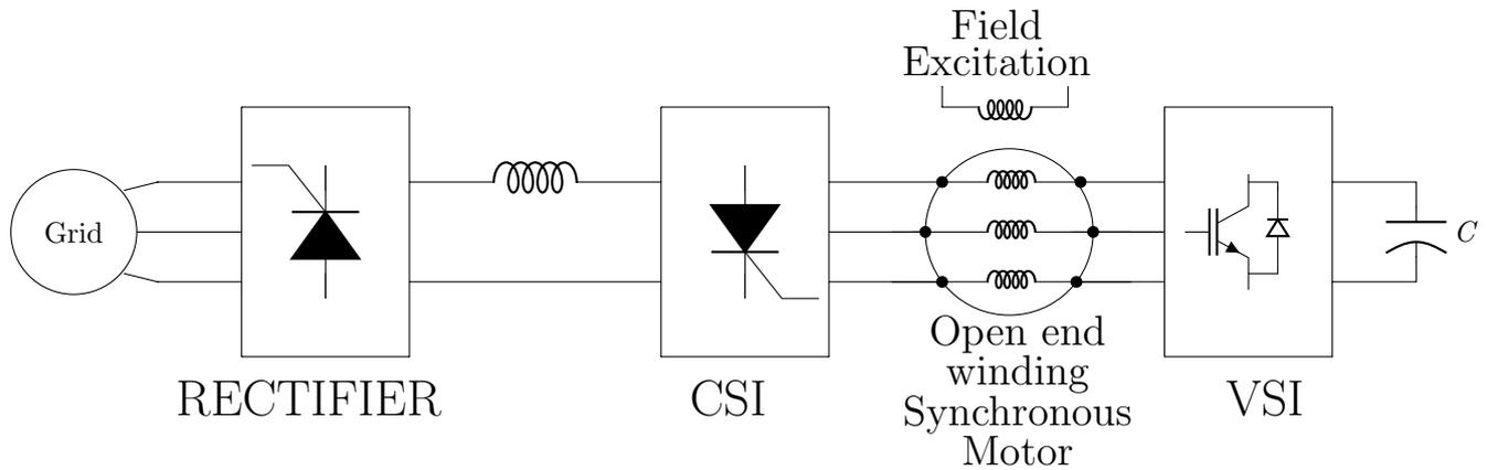
**Figure 4.1:** Block diagram of the proposed load commutated open-end winding synchronous motor drive.
