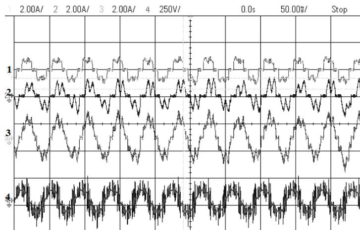
**Figure A.7:** Experimental results with multilevel CSI configuration : Motoring operation at 750 RPM: X-axis: 50ms/div. Ch-1: A-phase CSI-1 current (Y-axis: 2 A/div). Ch-2: A-phase CSI-2 current (Y-axis: 2 A/div) . Ch-3: A-phase motor current (Y-axis: 2 A/div). Ch-4: A-phase stator voltage of motor (Y-axis: 250 V/div).
