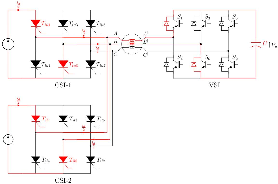
**Figure 3.15:** Pre-charging scheme for the capacitor of VSI.
