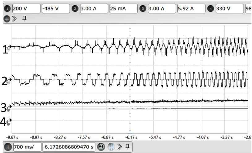
**Figure 4.12:** Experimental result for acceleration of motor from standstill state to 300 RPM: X-axis: 700 ms/div. Ch:1. Motor voltage (Y-axis: 200 V/div.). Ch:2. Motor current (Y-axis: 3 A/div.). Ch:3. DC-link current (Y-axis: 3 A/div.).Ch:4. VSI capacitor voltage (Y-axis: 330 V/div.).
