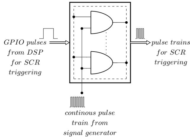
**Figure 5.8:** Block diagram of digital card for SCR gate pulse train generation.
