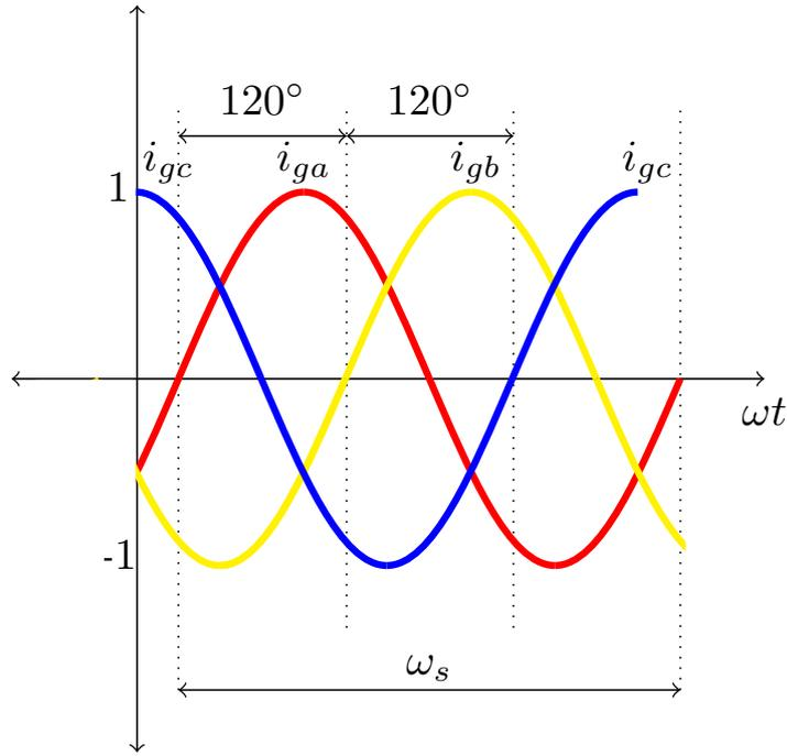
**Figure 2.12:** Unit magnitude three phase sinusoidal signals for CSI gate pulse generation
