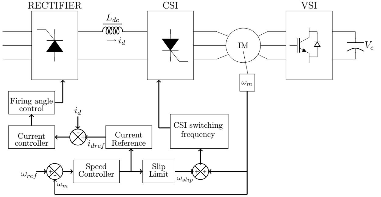
**Figure 2.13:** Implementation of CSI control scheme
