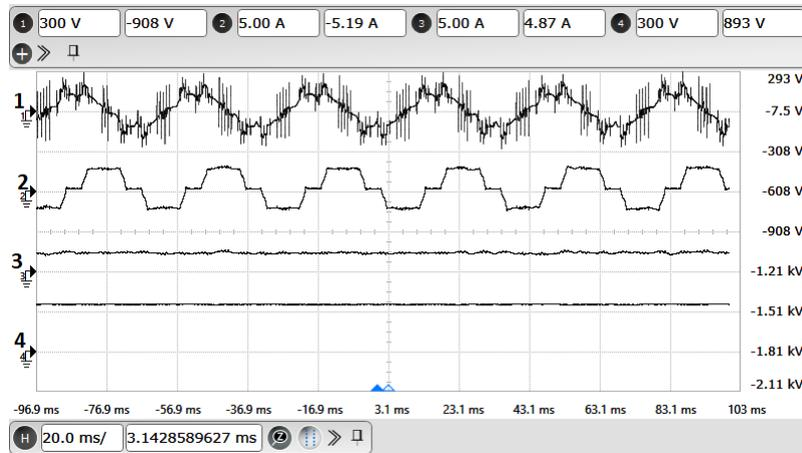
**Figure A.2:** Experimental results with single CSI configuration: Motor operation at 900 RPM : X-axis: 20 ms/div. Ch-1: A-phase stator voltage (Y-axis: 300 V/div). Ch-2: A-phase motor current (Y-axis: 5 A/div) . Ch-3: DC link current (Y-axis: 5 A/div) . Ch-4: VSI capacitor voltage (Y-axis: 300 V/div).
