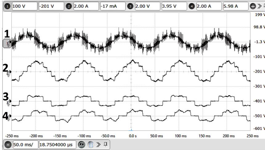
**Figure 3.27:** Experimental results: Motor operation at 300 RPM with multilevel CSI: X-axis: 50 ms/div. Ch-1: A-phase stator voltage of motor (Y-axis: 100 V/div). Ch-2: A-phase motor current (Y-axis: 2 A/div). Ch-3: A-phase CSI-1 current (Y-axis: 2 A/div). Ch-4: A-phase CSI-2 current (Y-axis: 2 A/div).
