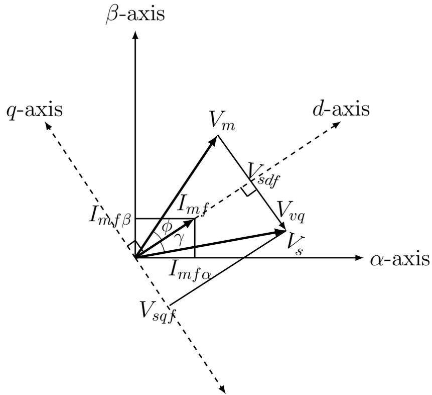
**Figure 2.15:** Phasor diagram showing the orientation of d-q axes, fundamental component of motor current ( $I_{mf}$ ) and CSI terminal voltage ( $V_s$ ).
