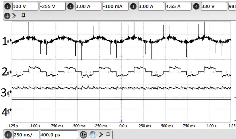
**Figure 4.9:** Experimental result at 75 RPM of motor operation: X-axis: 250 ms/div. Ch:1. Motor voltage (Y-axis: 100 V/div.). Ch:2. Motor current (Y-axis: 3 A/div.). Ch:3. DC-link current (Y-axis: 3 A/div.).Ch:4. VSI capacitor voltage (Y-axis: 330 V/div.).
