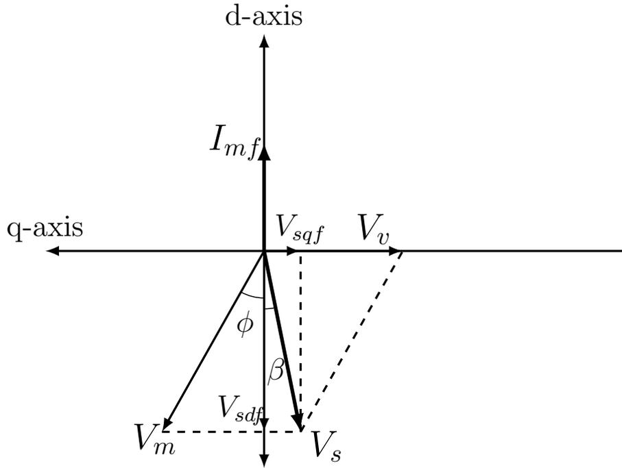
**Figure 3.14:** Phasor diagram during regeneration.
