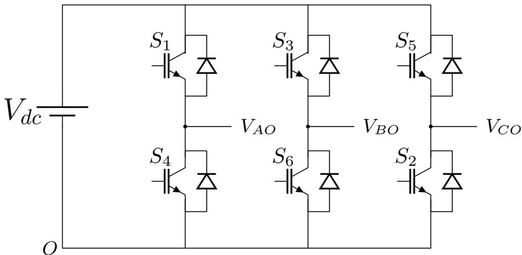
**Figure 1.5:** A three-phase inverter structure.
