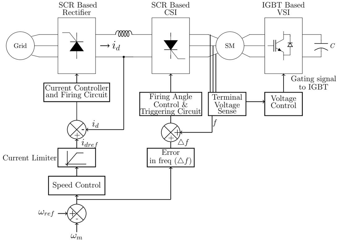
**Figure 4.5:** Synchronous motor speed control scheme.
