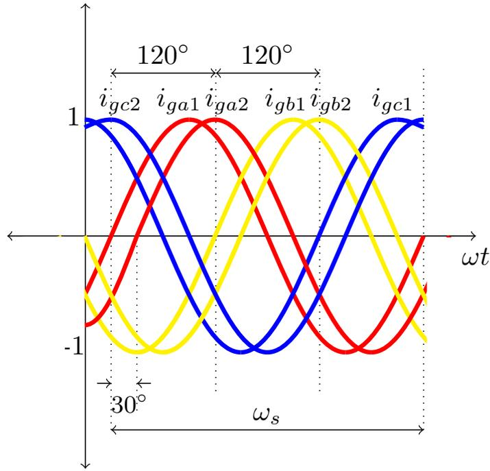
**Figure 3.10:** Unit magnitude three phase sinusoidal signals for SCR firing pulse generation of CSI-1 and CSI-2.
