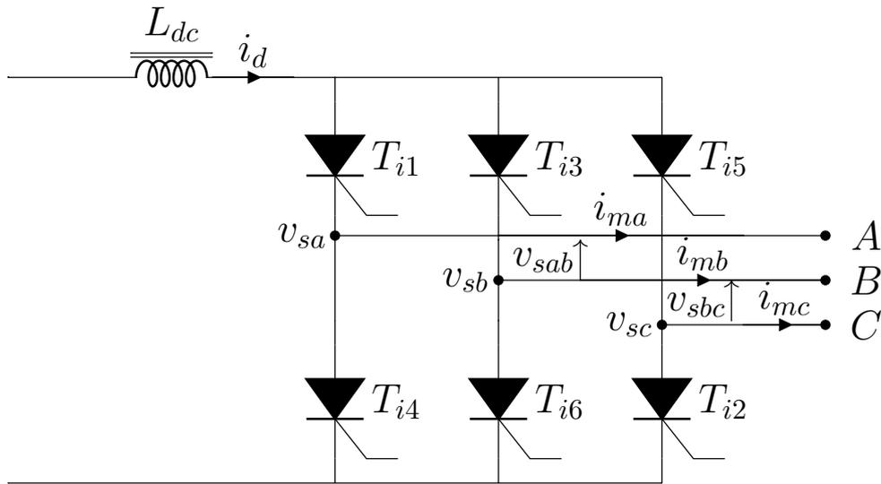
**Figure 2.5:** Circuit diagram of load commutated SCR based CSI.
