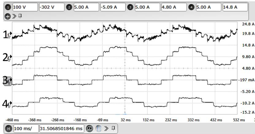
**Figure 3.24:** Experimental results during low speed operation at nearly rated torque (100 RPM): X-axis: 100 ms/div. Ch-1: A-phase stator voltage of motor (Y-axis: 100 V/div). Ch-2: A-phase motor current (Y-axis: 5 A/div). Ch-3: A-phase CSI-1 current (Y-axis: 5 A/div). Ch-4: A-phase CSI-2 current (Y-axis: 5 A/div).
