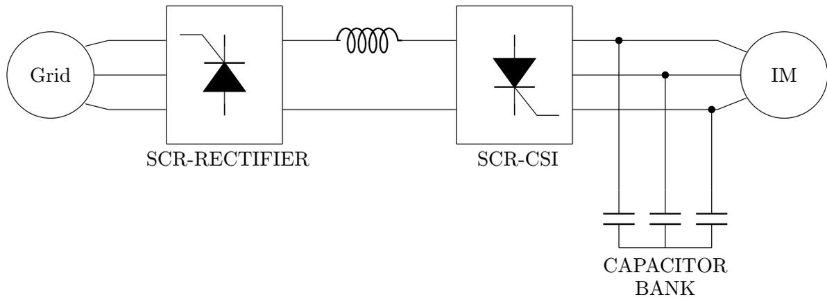
**Figure 1.11:** Block diagram of load commutated IM drive with capacitor bank.
