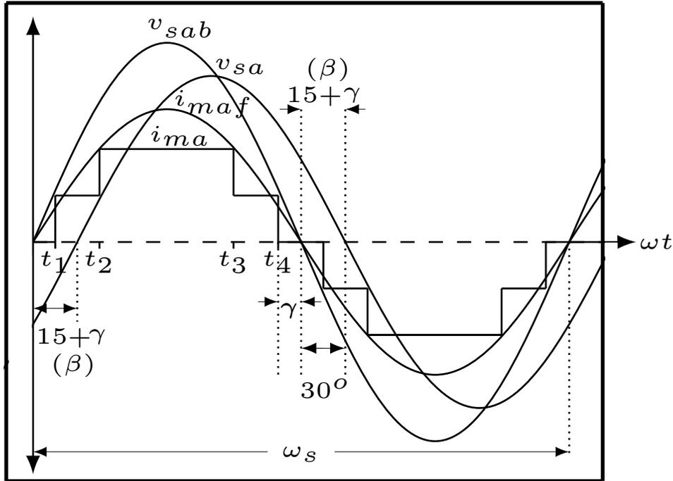
**Figure 3.7:** Waveforms of CSI line voltage ( $v_{sab}$ ), CSI terminal voltage ( $v_{sa}$ ), motor current ( $i_{ma}$ ) and its fundamental component ( $i_{maf}$ ) during motoring operation.
