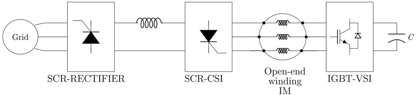
**Figure 1.14:** Block diagram of the proposed scheme of load commutated SCR based CSI fed IM drive with open end stator windings.
