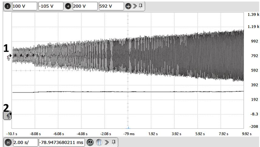
**Figure 3.22:** Experimental results : Acceleration of motor from 300 to 1000 RPM: X-axis: 2 s/div. Ch-1: A-phase stator voltage of motor (Y-axis: 100 V/div). Ch-2: VSI capacitor voltage  $V_c$  (Y-axis: 200 V/div).
