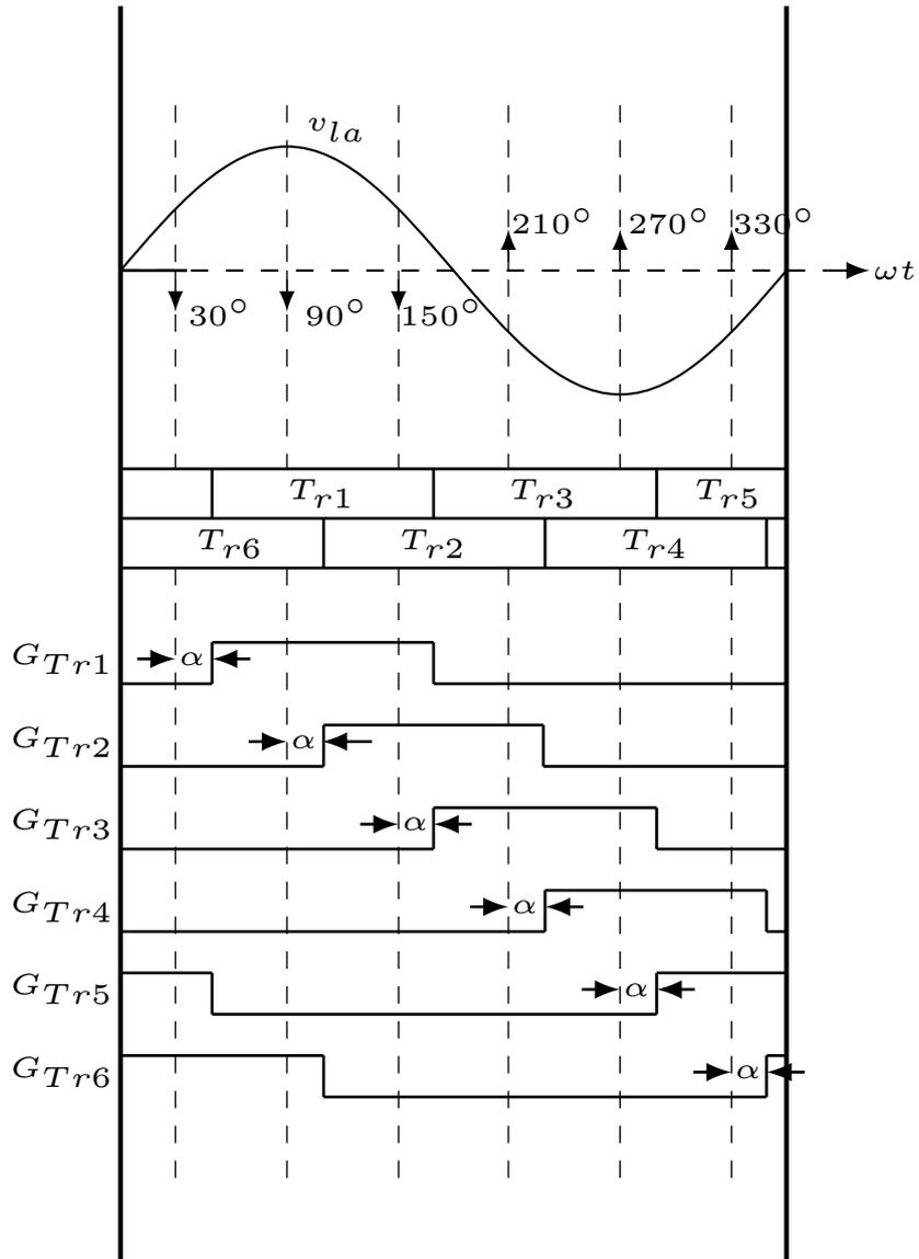
**Figure 2.4:** Rectifier SCR gating pulse pattern.
