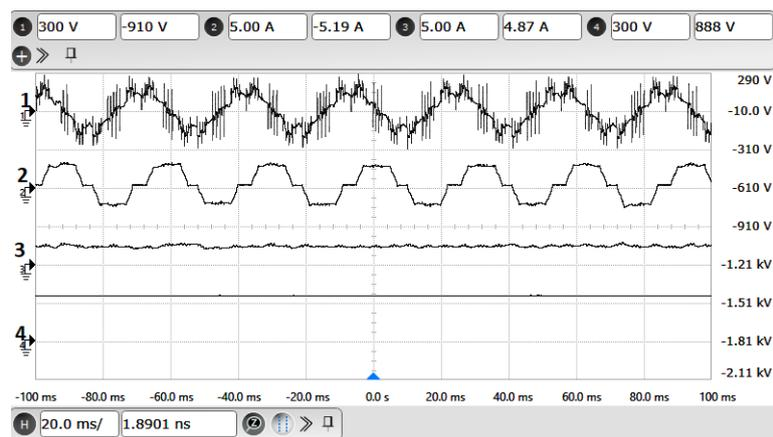
**Figure A.1:** Experimental results with single CSI configuration: Motor operation at 1000 RPM : X-axis: 20 ms/div. Ch-1: A-phase stator voltage (Y-axis: 300 V/div). Ch-2: A-phase motor current (Y-axis: 5 A/div) . Ch-3: DC link current (Y-axis: 5 A/div) . Ch-4: VSI capacitor voltage (Y-axis: 300 V/div).
