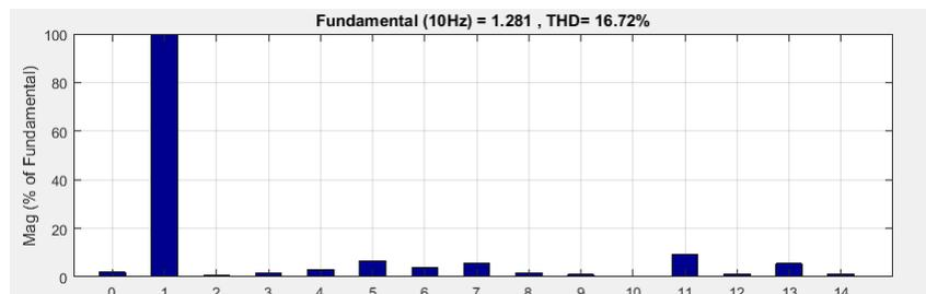
**Figure 3.28:** Harmonic spectrum of the motor current with multilevel CSI operation : X-axis (Harmonic order). Y-axis: (Magnitude in % of fundamental).
