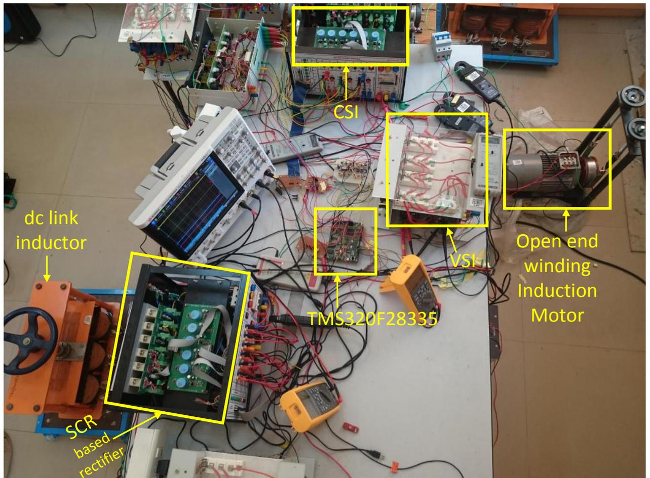
**Figure 2.19:** Photograph of the experimental setup
