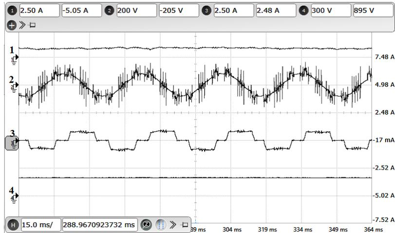
**Figure 2.22:** Experimental results: Motor operation at 900 RPM : X-axis: 15 ms/div. Ch-1: DC link current (Y-axis: 2.5 A/div). Ch-2: A-phase stator voltage(Y-axis: 200 V/div). Ch-3: A-phase motor current (Y-axis: 2.5 A/div). Ch-4: VSI capacitor voltage (Y-axis: 300 V/div).
