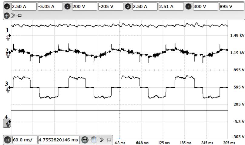
**Figure 2.20:** Experimental results: Motor operation at 200 RPM : X-axis: 60 ms/div. Ch-1: DC link current (Y-axis: 2.5 A/div). Ch-2: A-phase stator voltage(Y-axis: 200 V/div). Ch-3: A-phase motor current (Y-axis: 2.5 A/div). Ch-4: VSI capacitor voltage (Y-axis: 300 V/div).
