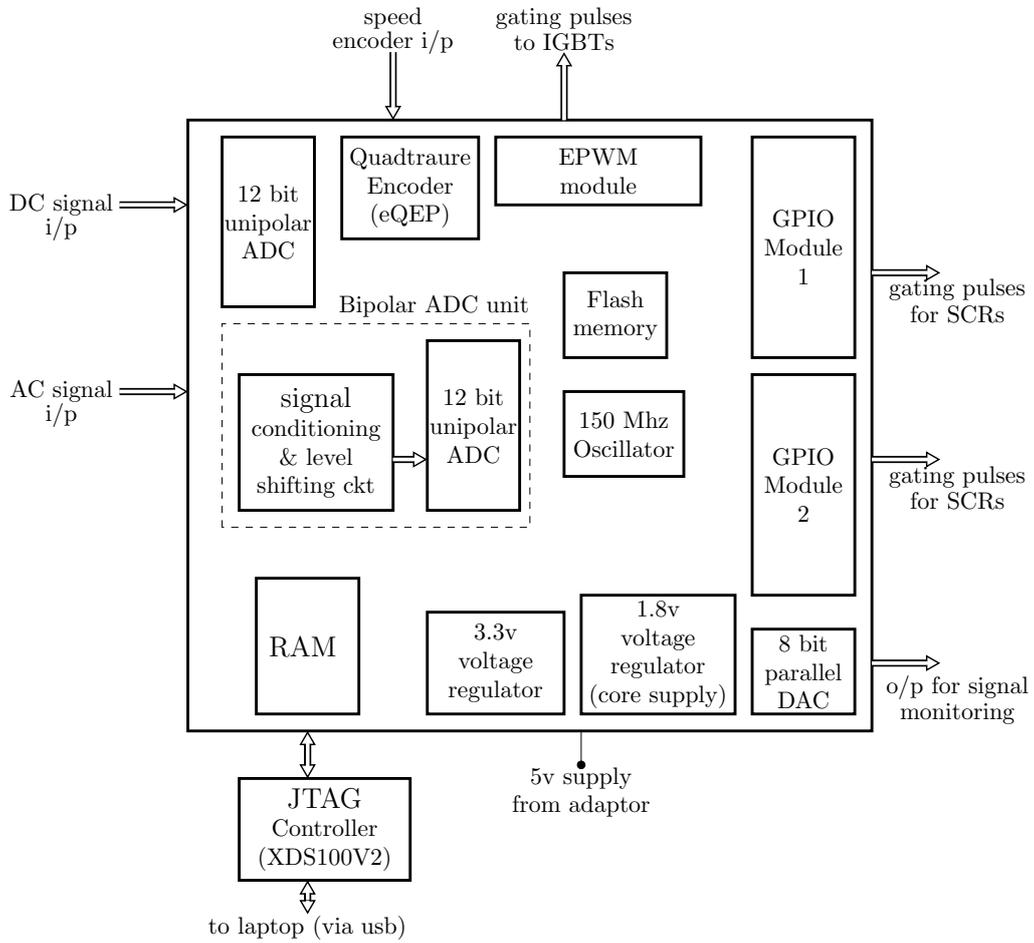
**Figure 5.6:** Block diagram of DSP board.
