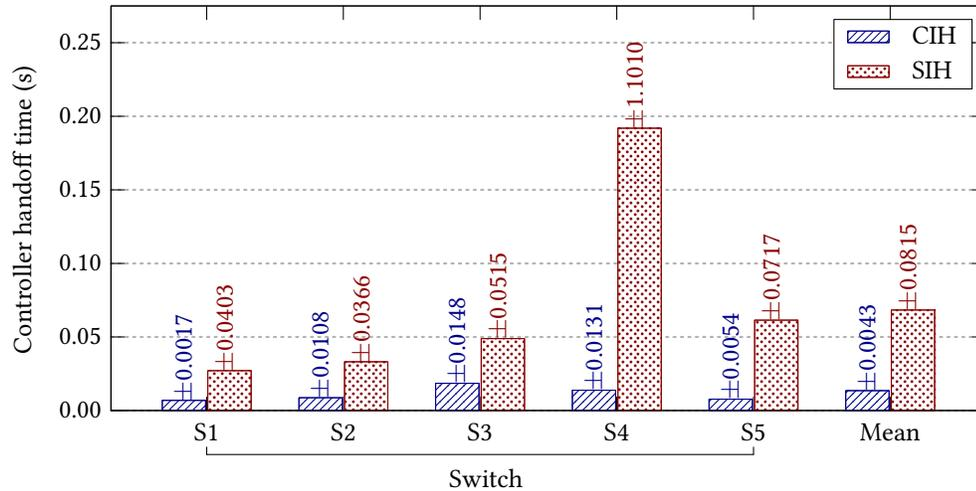
**Figure 3.19:** Controller handoff time. The standard deviation is provided on the top of each bar.
