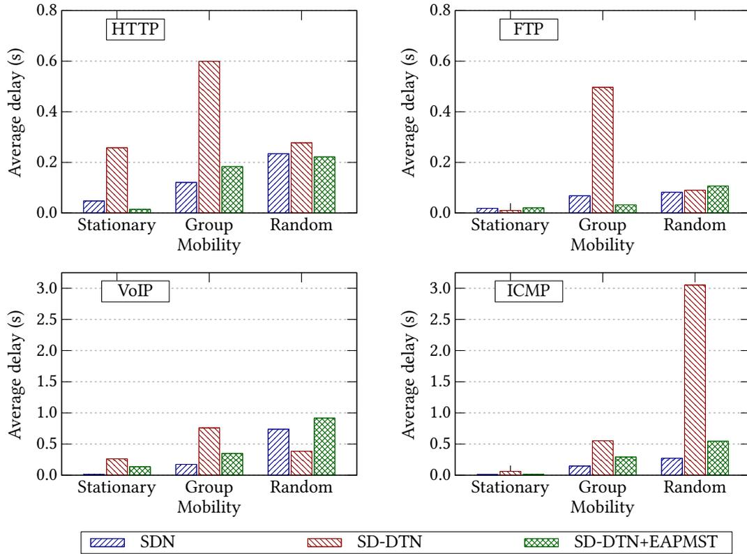
**Figure 4.12:** Average end-to-end delay incurred by the packets of the four communication protocols with the three SDN schemes under different mobility patterns.
