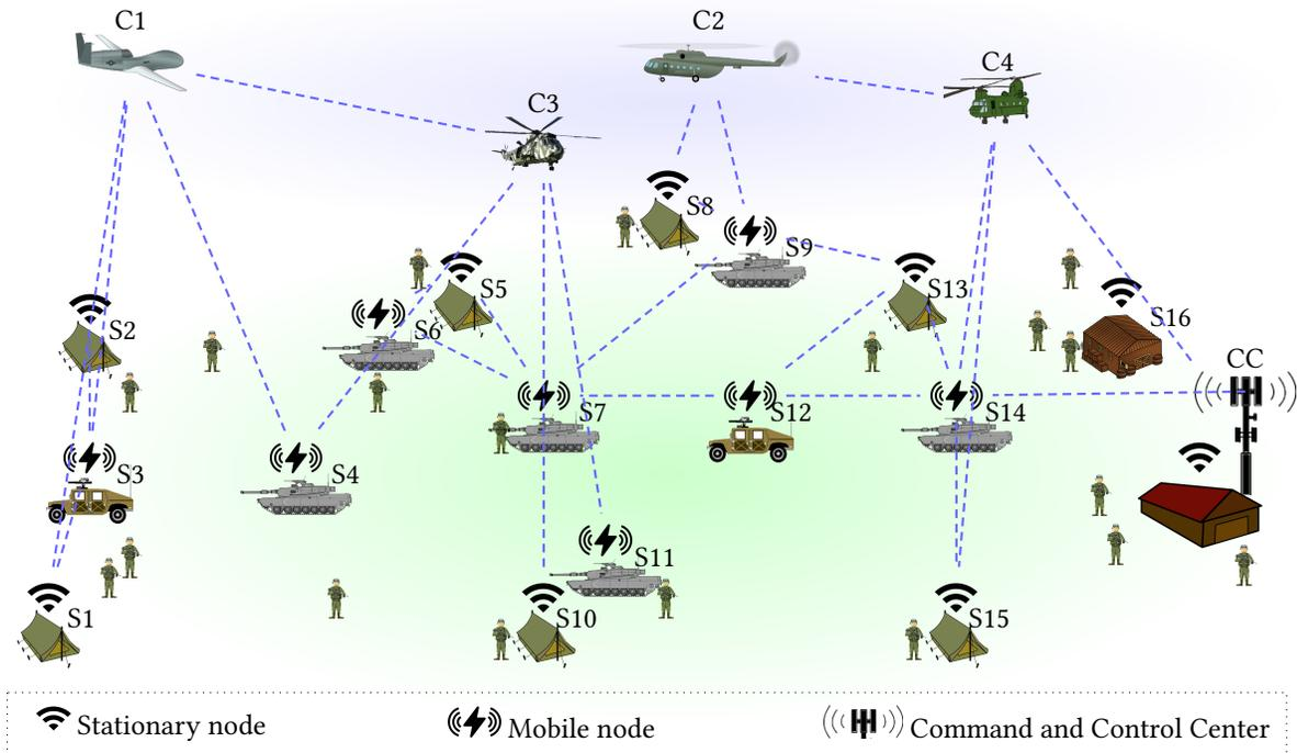
**Figure 5.20:** An example software defined tactical network scenario. The notations starting with the letter ‘C’ represent SDN controllers and those starting with the letter ‘S’ represent the switches.
