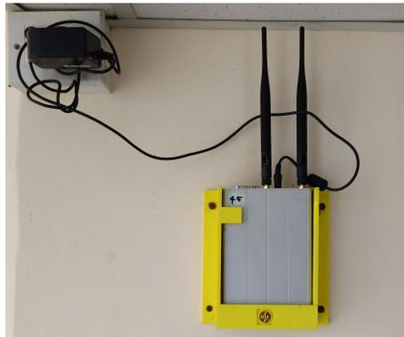
(a) Fixed switch mounted on the wall.
