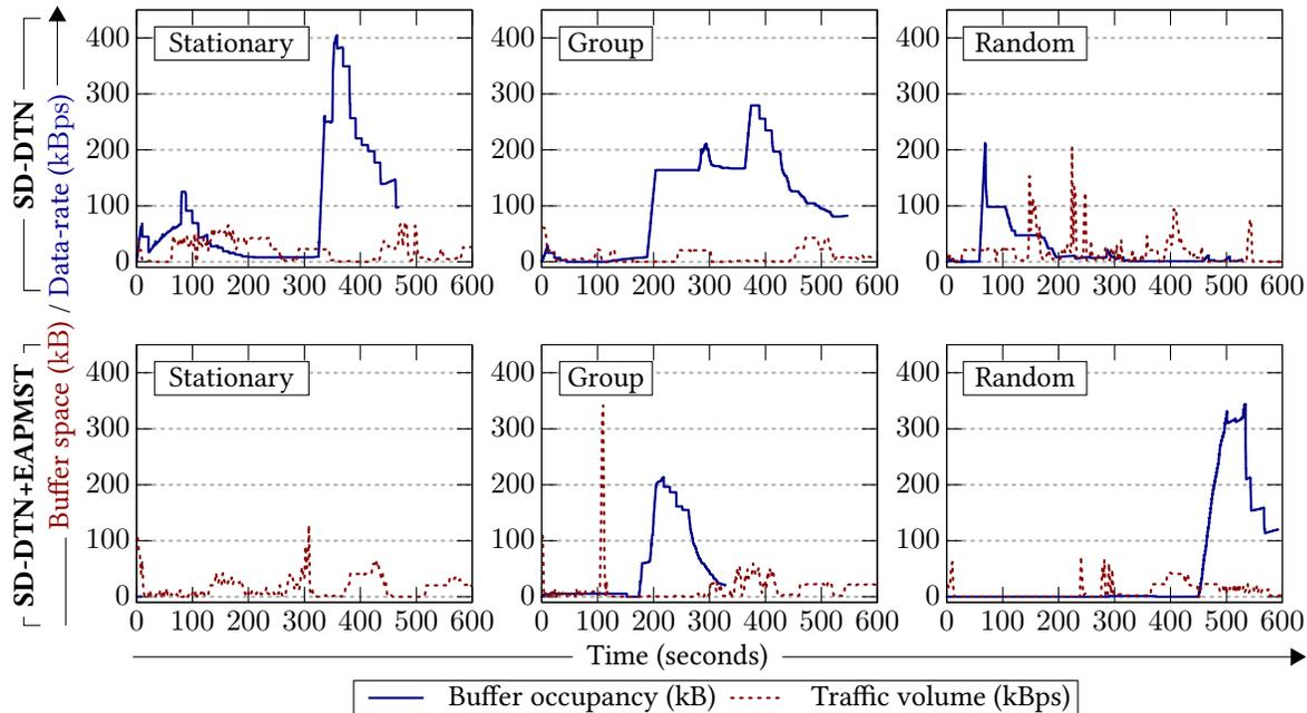
**Figure 4.18:** Buffer occupancy corresponding to the traffic volume through the timeline of the experiment on the most central node of the network.
