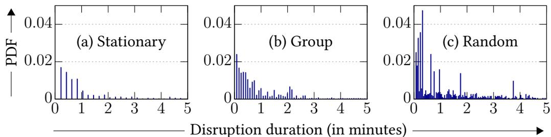
**Figure 1.8:** Distribution of link-disruption durations, represented as Probability Density Function (PDF), in a campus-based IISTMeshNet WMN testbed involving 32 nodes.
