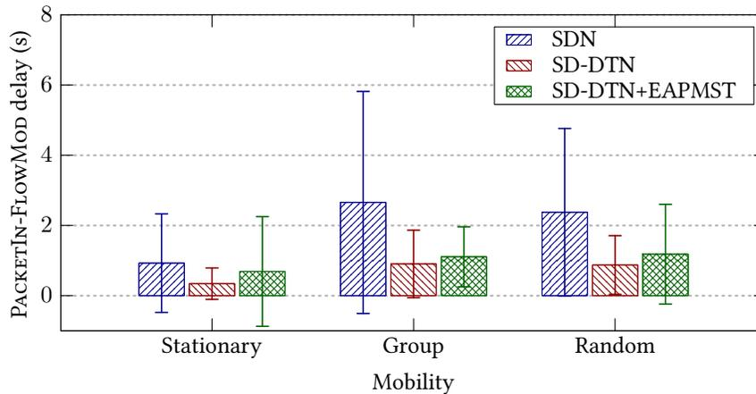
**Figure 4.11:** Average delay incurred in SDN control channel for the flow-rule request (PACKETIN) and response (FLOWMOD) packets.
