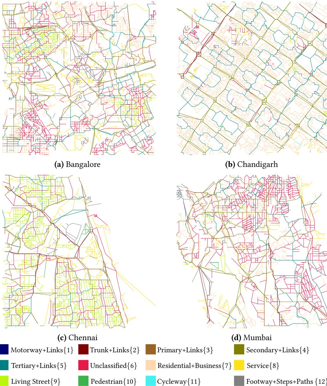
**Figure 5.4:** City road networks from India with dimension  $5 \text{ km} \times 5 \text{ km}$  around the city center. The color code represents 12 classes of road-types and the type-value of each road-type is given within braces.
