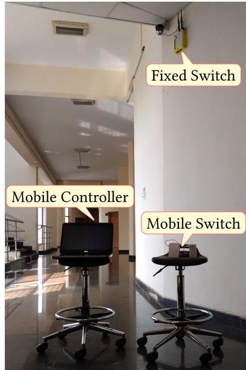
(c) Fixed switch, mobile switch, and mobile controller.
