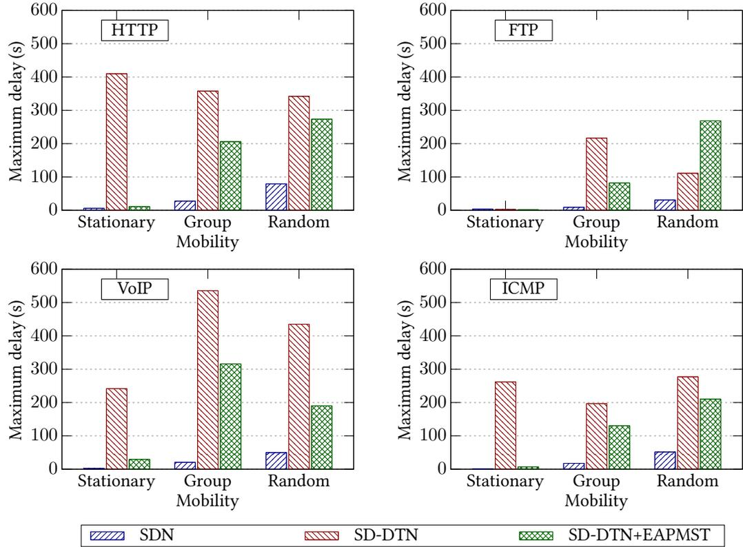
**Figure 4.13:** Maximum end-to-end delay incurred by packets of the four protocol sessions with the three SDN schemes under different mobility pattern of nodes.
