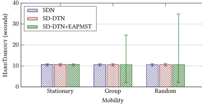
**Figure 4.15:** HARDTIMEOUT values provided by the three SDN control schemes under different mobility models considered. The error lines indicate the minimum and maximum values of the HARDTIMEOUT value, not the standard deviation.
