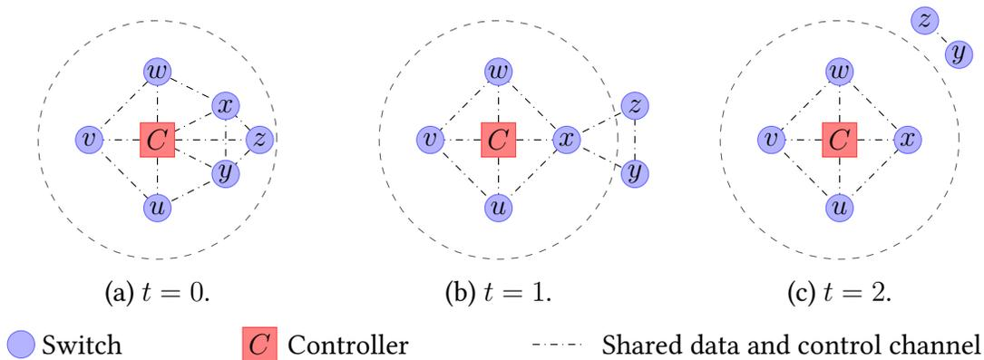
**Figure 1.4:** Control channel operating in in-band mode. The dashed circle depicts the communication range of the controller.
