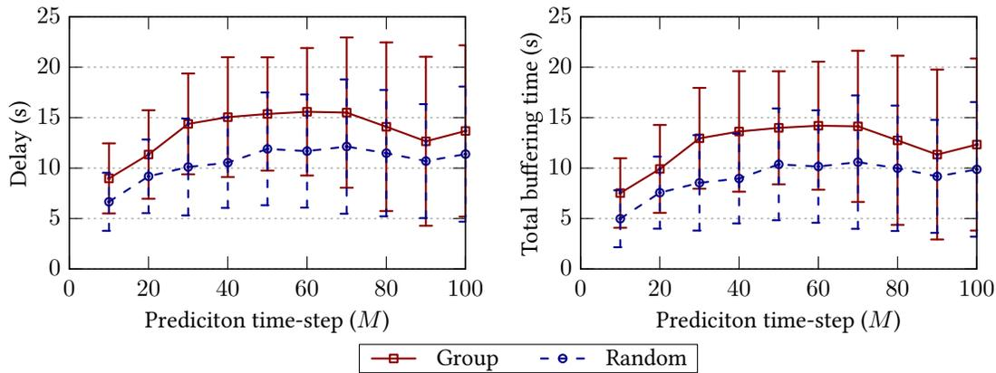
**Figure 4.21:** End-to-end delay and the corresponding buffering time achieved by SD-DTN with the default buffering time of  $M$  seconds.
