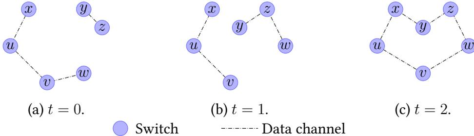
**Figure 1.5:** Example disruption tolerant networking scenario in data plane.
