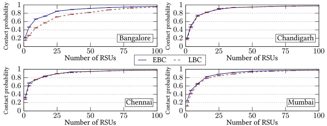
**Figure 5.6:** Contact probability under the shortest path traffic based on minimum travel time.
