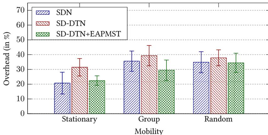
**Figure 4.14:** OpenFlow overhead on the network in the three SDN control schemes under different mobility models.
