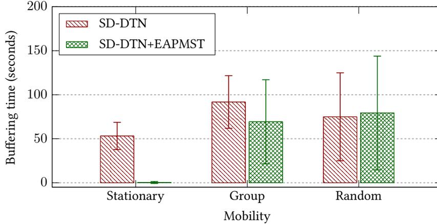
**Figure 4.16:** Buffering time incurred by packets in SD-DTN-based control schemes.
