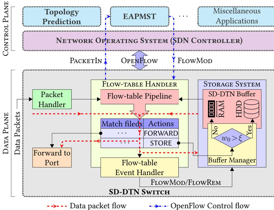
**Figure 4.5:** A new architecture for SD-DTN switch and its interaction with the SDN controller. The Red dashed lines show the flow of data packets within the switch while the Blue dash-dotted lines show the flow of SDN control packets between switch and the controller.
