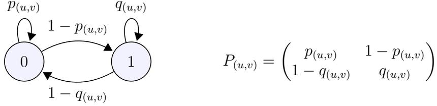
**Figure 4.2:** State-transition diagram and the corresponding transition probability matrix of an edge  $(u, v)$ .
