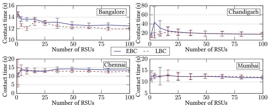
**Figure 5.7:** Contact time under the shortest path traffic based on minimum travel time.
