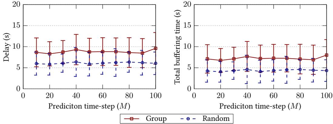
**Figure 4.20:** End-to-end delay and the corresponding buffering time achieved by SD-DTN with the default buffering time of 10 seconds.
