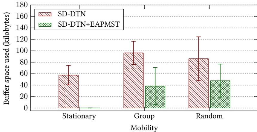
**Figure 4.17:** Buffer space occupied by SDN control schemes under the three mobility models.
