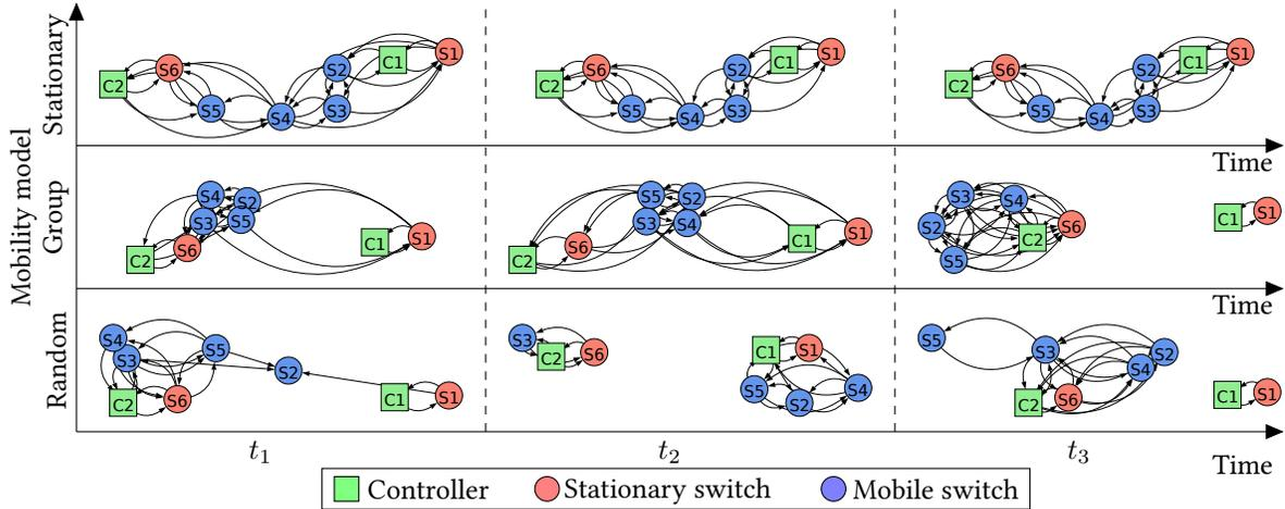
**Figure 4.7:** Snapshots of network topology from the three mobility models during the experiment timeline.
