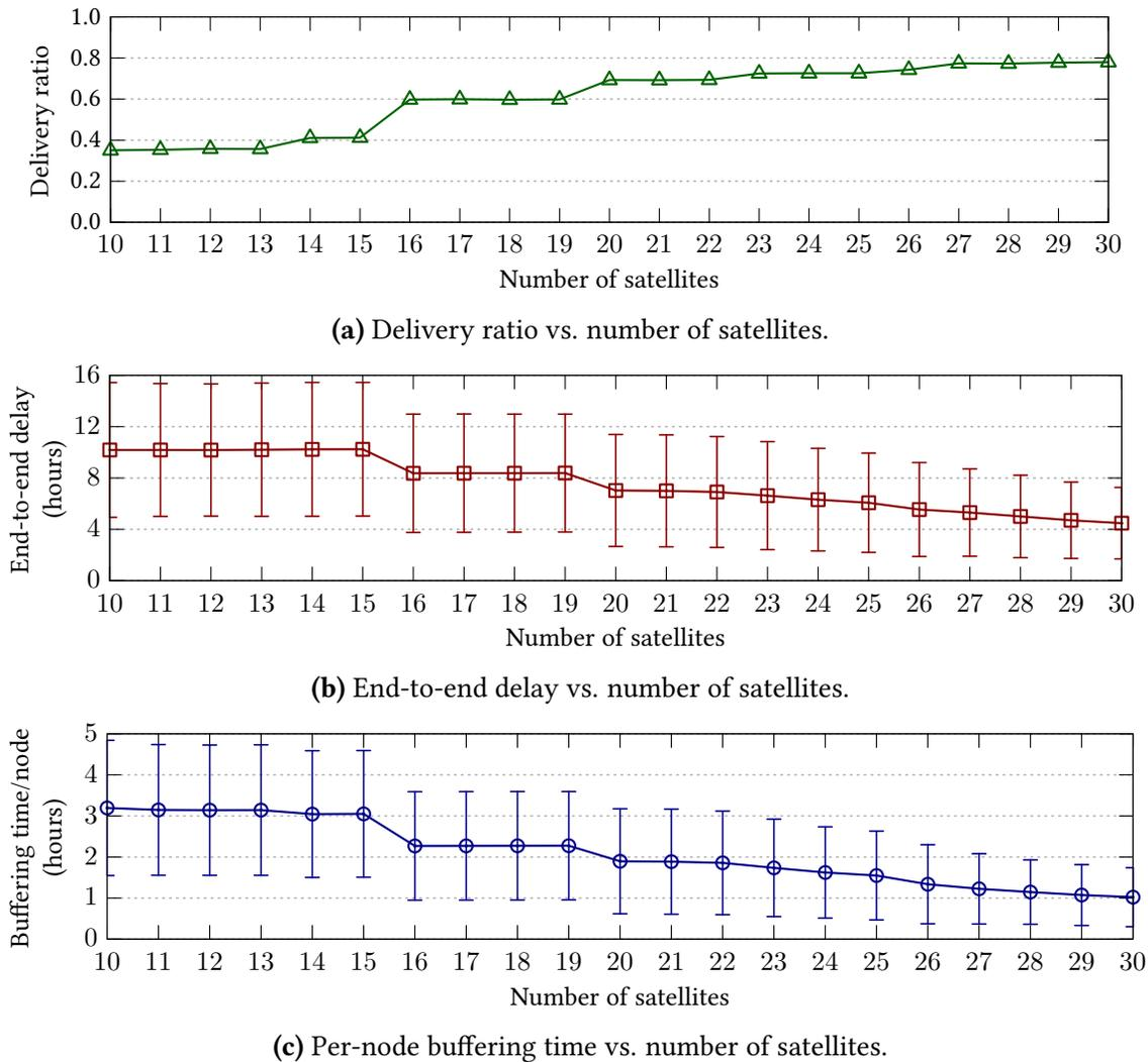
**Figure 5.19:** Performance of EAPMST on DebrisNet with varying number of satellites.
