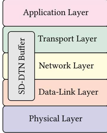
**Figure 4.4:** Protocol stack for the SD-DTN switch with a dedicated buffer for controlled buffering.
