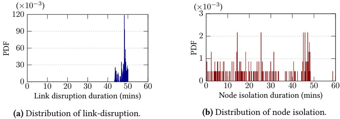
**Figure 5.13:** The distribution of durations of link disruptions and node isolation in *Constrained-Iridium-NEXT* constellation. The distribution is represented using probability density functions.
