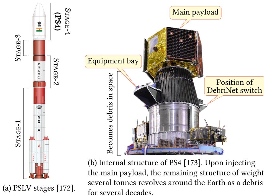
**Figure 5.15:** Stages of PSLV and the internal structure of PS4 module.
