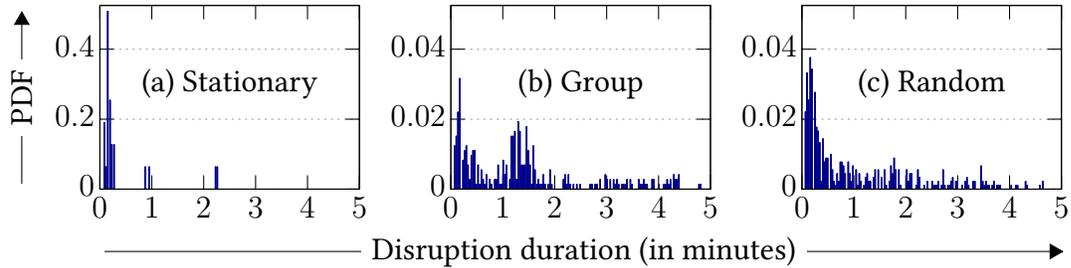
**Figure 4.8:** Distribution of link disruption durations, represented as Probability Density Functions (PDFs), from our experiments in SD-DTN testbed corresponding to the three mobility models.
