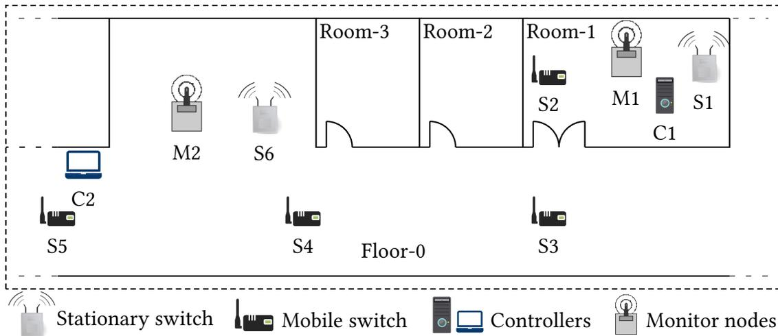
**Figure 4.6:** Layout of the SD-DTN testbed from Floor-0 of the IIST Avionics Department Building.
