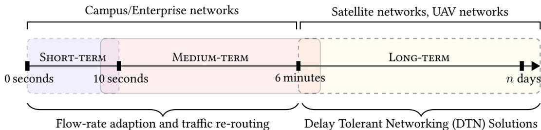
**Figure 4.1:** Classification of link disruptions based on disruption duration.
