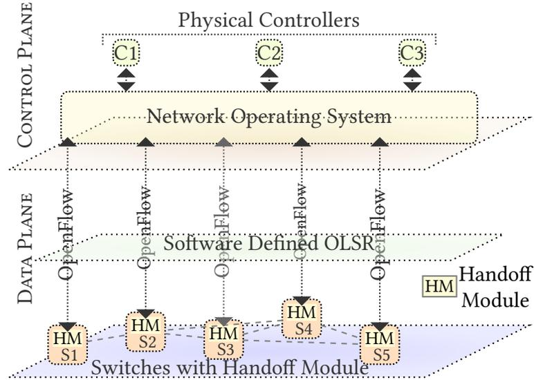
**Figure 3.2:** Architecture of switch-initiated handoff.
