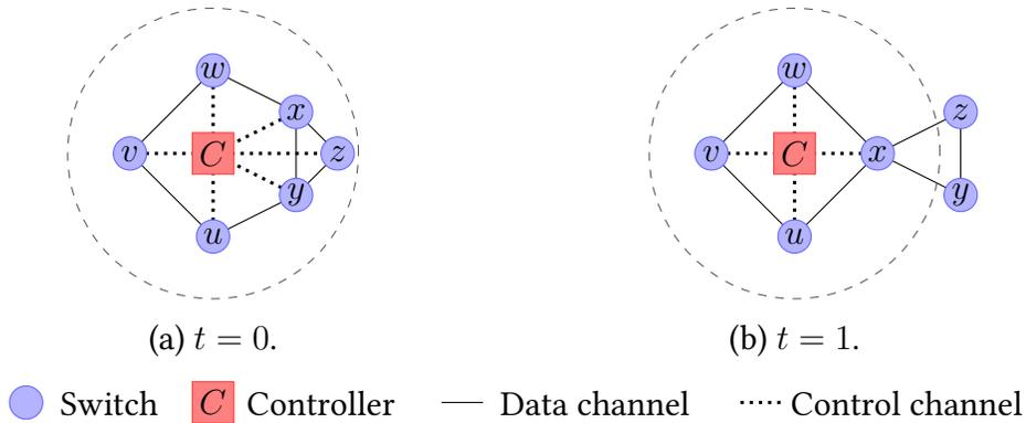
**Figure 1.3:** Control channel operating in out-of-band mode. The dashed circle depicts the communication range of the controller.
