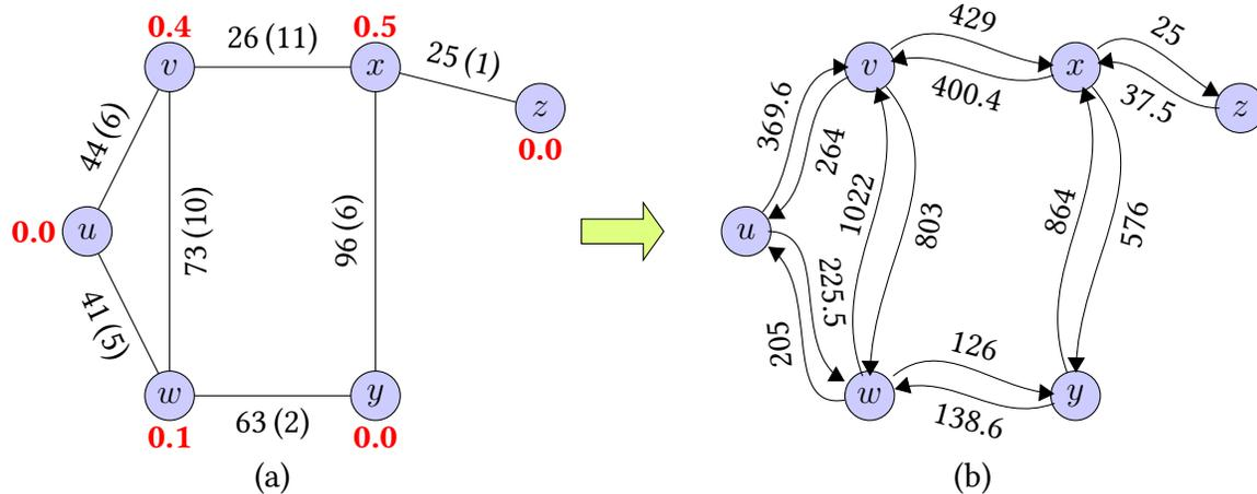
**Figure 5.3:** (a) An example graph  $G$  with six junctions. The length of each link is notated beside the link along with the road-type specified within brackets. The BC value of each junction is provided near the junction in bold face. (b) *Effort-graph* with links weighted with their corresponding *Effort*.
