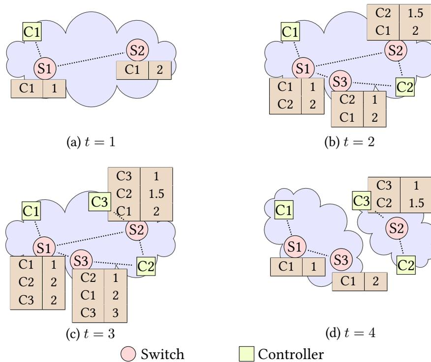
**Figure 3.4:** Snapshots of an SD-WMN running SD-OLSR protocol. The candidate controller table associated with each switch is provided near the switch.
