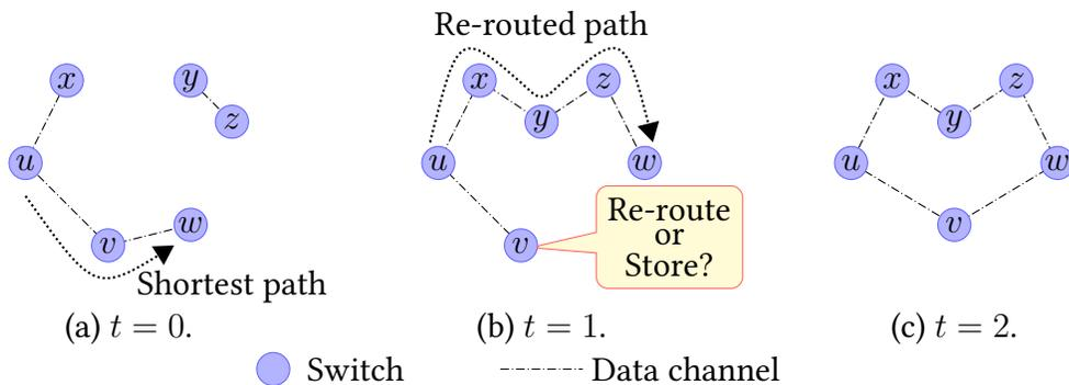
**Figure 1.9:** An example WMN involving link disruptions. The time (cost) required for each link to carry the packets is assumed to be 1 second.
