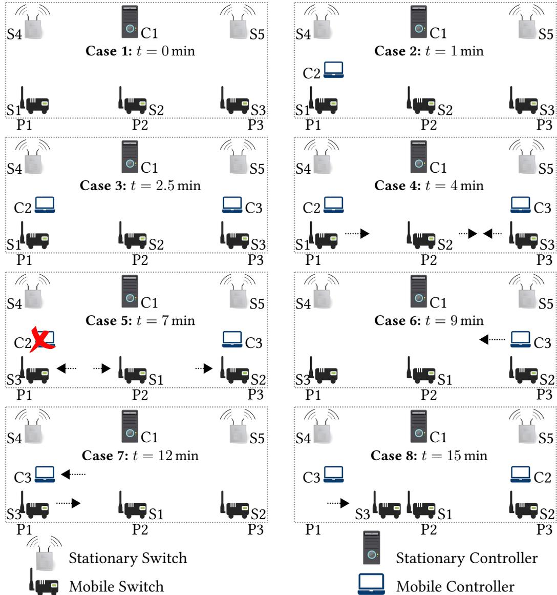
**Figure 3.6:** Experiment sequence involving mobility of switches and controllers.
