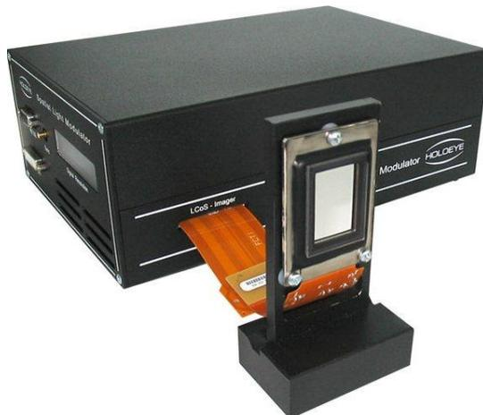
Figure A3.2: Photograph of LC-R 720 SLM
