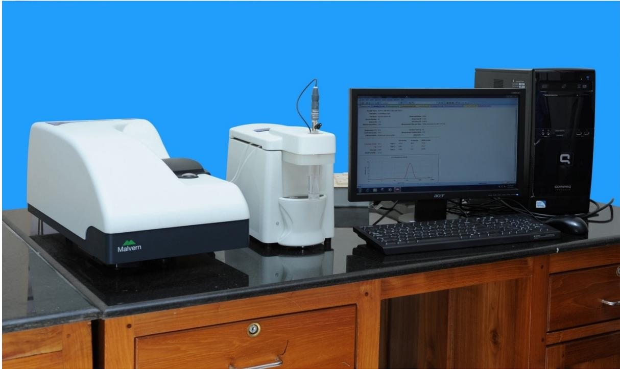
**Figure 3.5:** Zetasizer-Nano for particle size measurement using DLS technique
