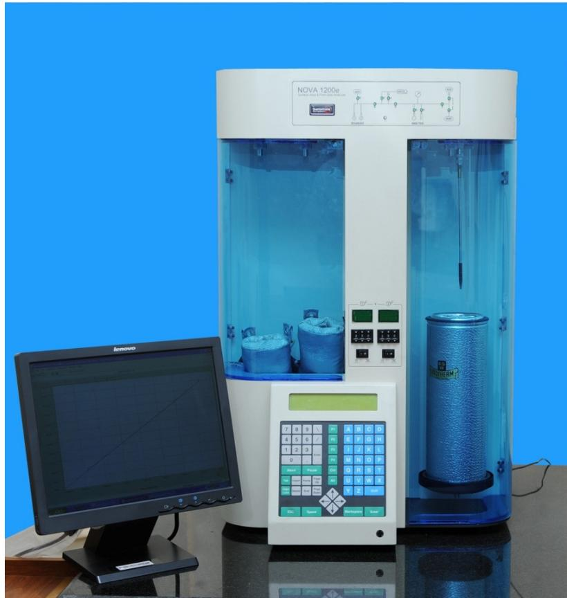
**Figure 3.3:** Instrument for particle specific surface area measurement
