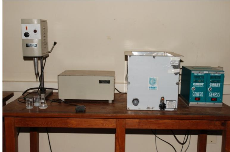
**Figure 3.1:** Ultrasonic disruptor and bath (25KHz 500W)
