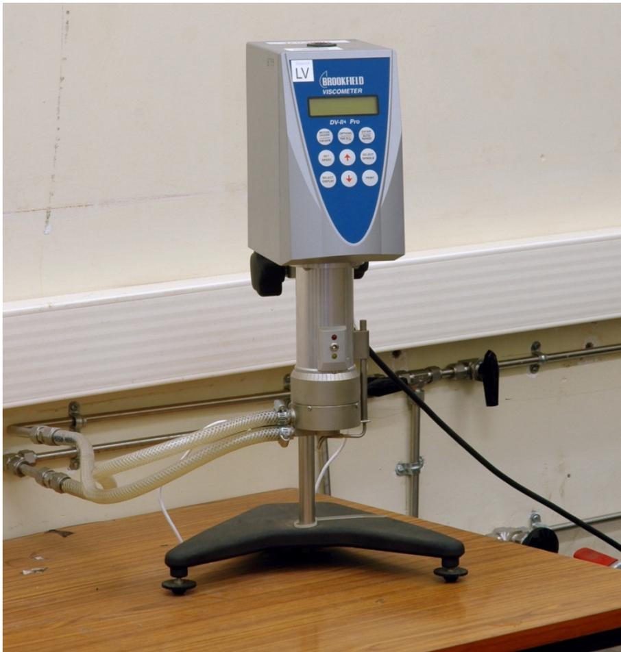
**Figure 3.8:** Brookfield LVDV-II for viscosity measurements
