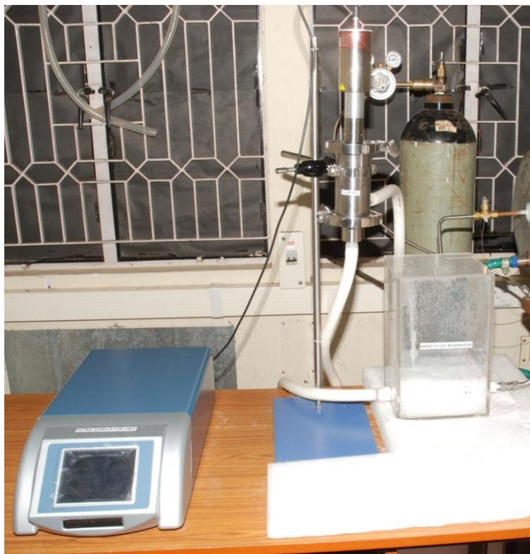
**Figure 3.2:** Ultrasonic disruptor with flow cell
