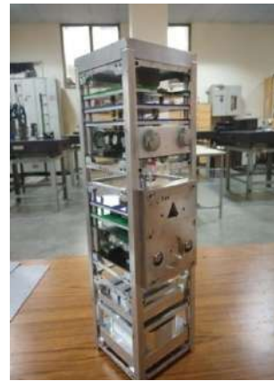
Figure: Mirrorsat Mass dummy of IIST delivered to Caltech for integration and testing
