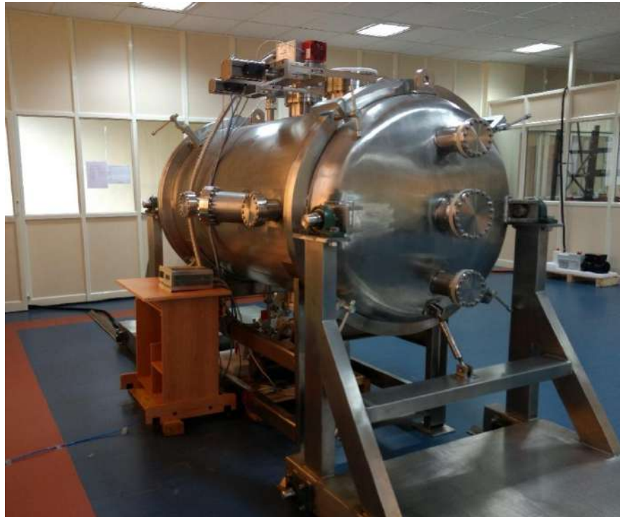
Figure 1 1 m X 1.5 class High Vacuum chamber at EPDL, IIST
