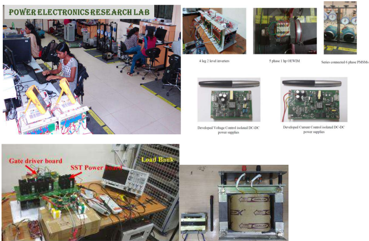
1.5 kVA SST prototype developed inhouse at PEDS Lab Comparison: 1.5 kVA HFAC (left) with normal 50 Hz transformer
